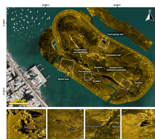
Figure 5. Side scan sonar mosaic map of the study area showing the traces of the submerged ancient harbor. (a) Very-coarse boulders; (b) Coarse boulders; (c) Buried archaeological remains; (d) Outcropping reefs.
