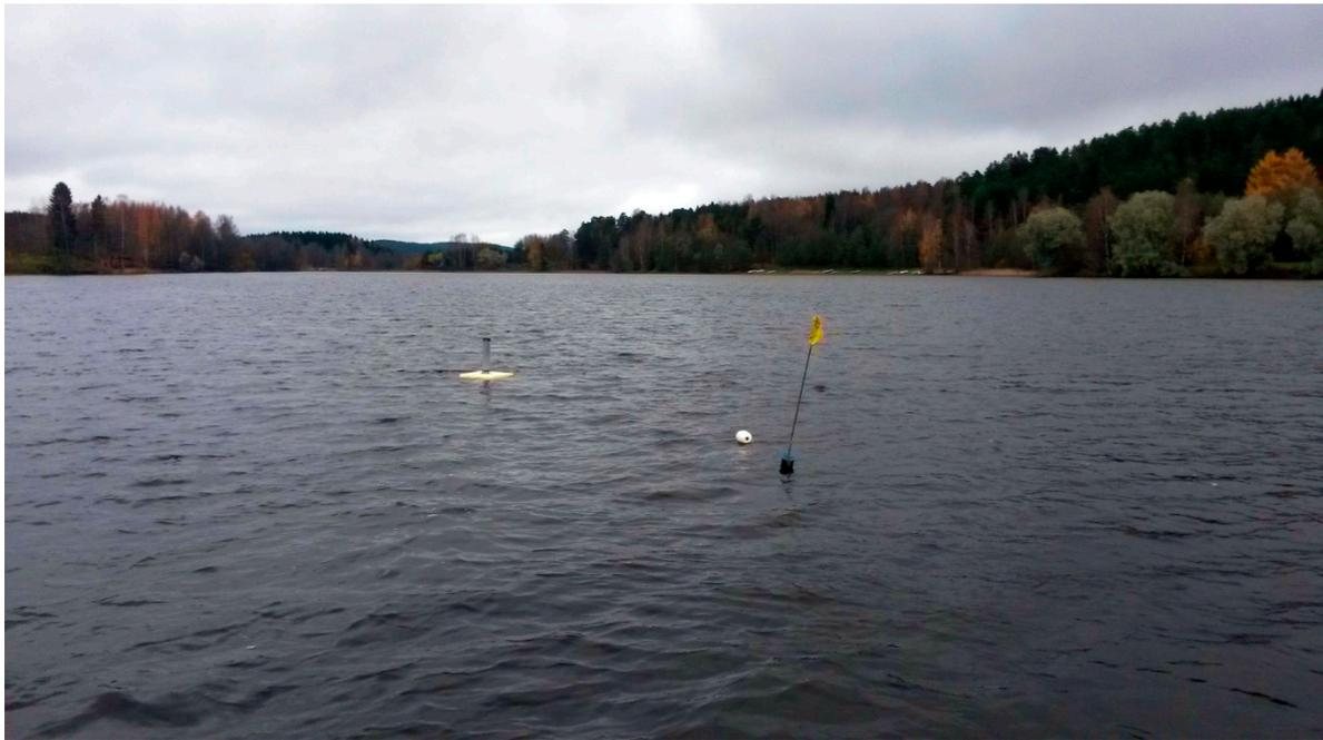
**Figure 3.** Online trap in Savilahti Bay basin at a depth of 6 m under the flag sign. Anchored float behind flag sign is the base station for the online trap, which sends measurements to the Internet over a mobile network.
