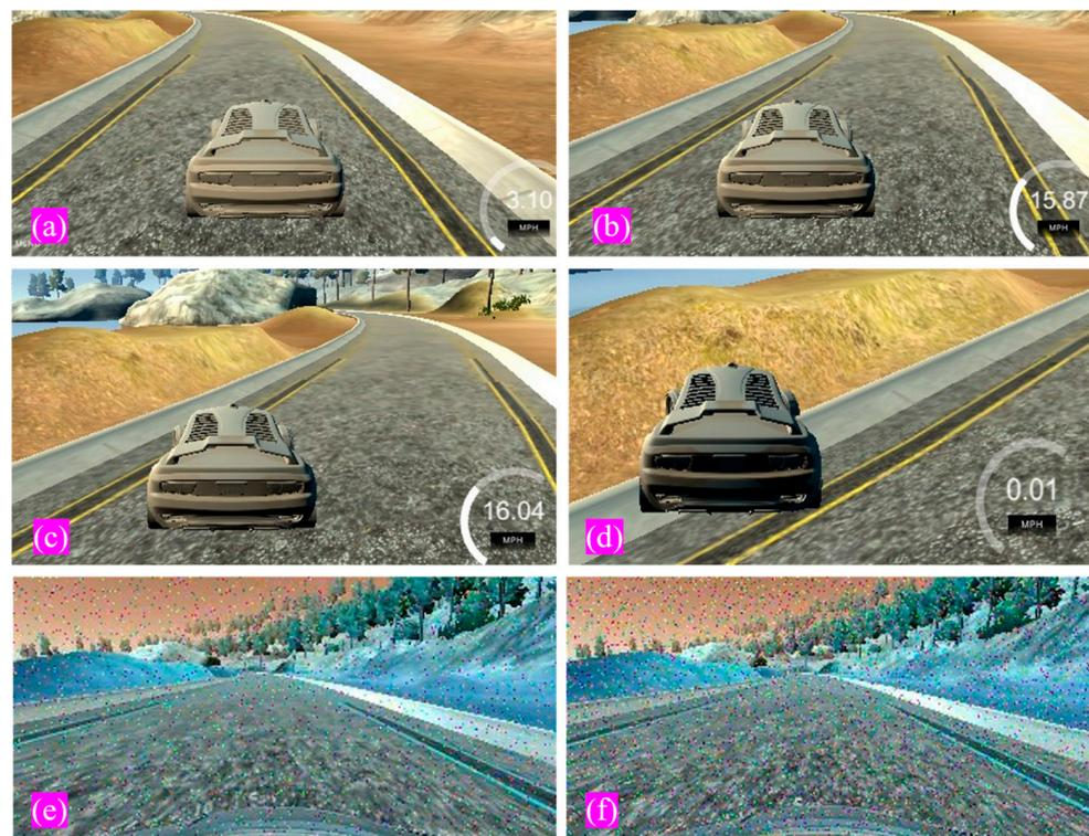
**Figure 3.** Impact of adversarial attack on the original trajectory of the target ADS. These samples were collected when the impulse-noise-based adversarial attack was applied. (a) represents the initial position, and (b,c) show the impact of the attack. We can see that the ADS started deviating from its original trajectory. (d) shows that ADS is no longer driving on the road and crashed on the roadside. (e,f) represents the samples of adversarial image frames from front camera of ADS.
