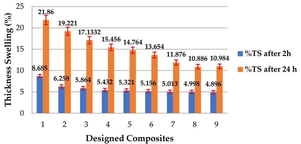
Figure 7. Variation in thickness swelling against board samples.
