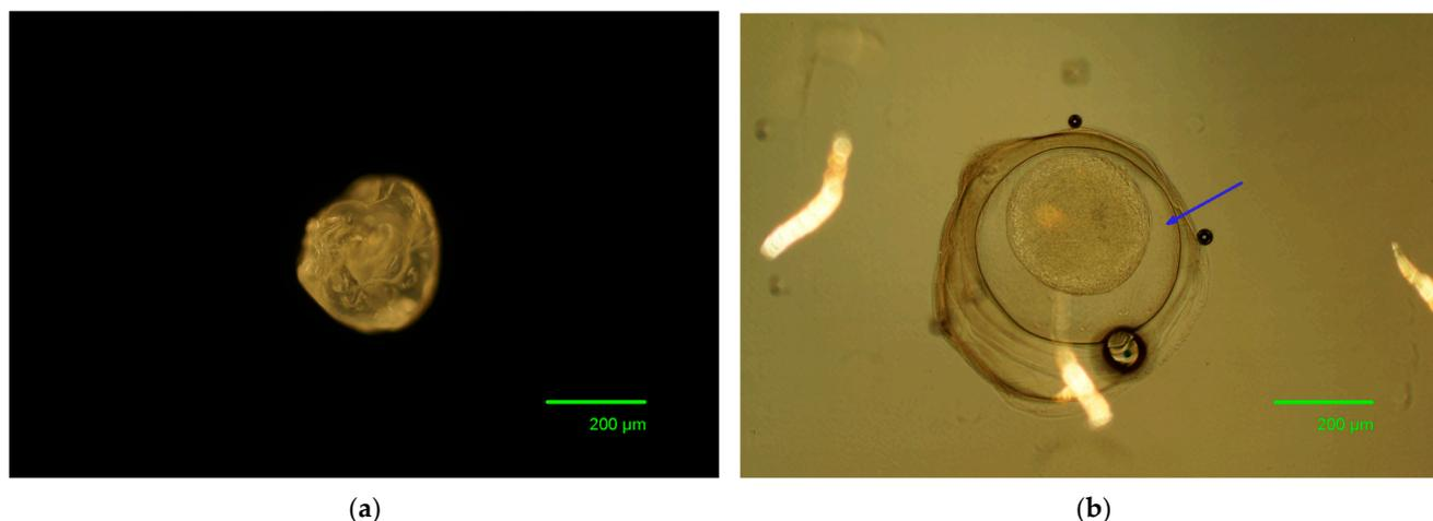
**Figure 6.** Microscopic images of a composite particle (a) in the dried state (3 d drying above silica-gel; dark field image) and (b) 80 min after subsequent immersion in water (transmitted light with polarization filter; arrow indicates the void between the core and shell). Core—2% agarose 4018 + 1% gelatin G9391 + 27% trehalose; shell—NIPAM 0.85 M + AA 0.12 M + BDDA 0.062 M.
