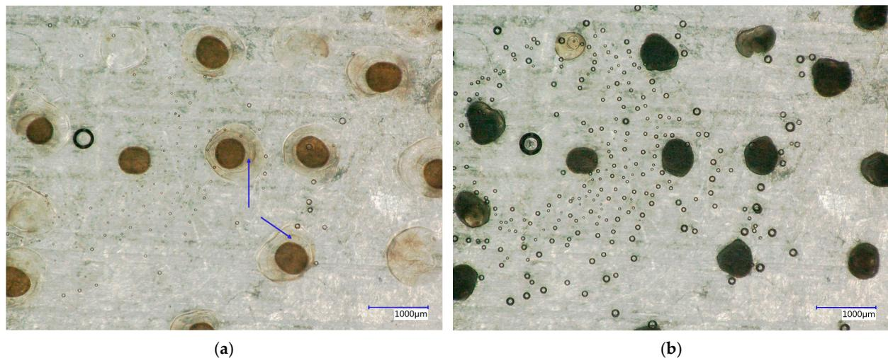
**Figure 3.** Microscopic images of composite particles with shells of PNIPAM crosslinked with MBBA (a) at 26 °C and (b) 38 °C, respectively. NIPAM 0.93 M, MBBA 0.076 M, and dark agarose cores; arrows indicate the voids between the core and shell.
