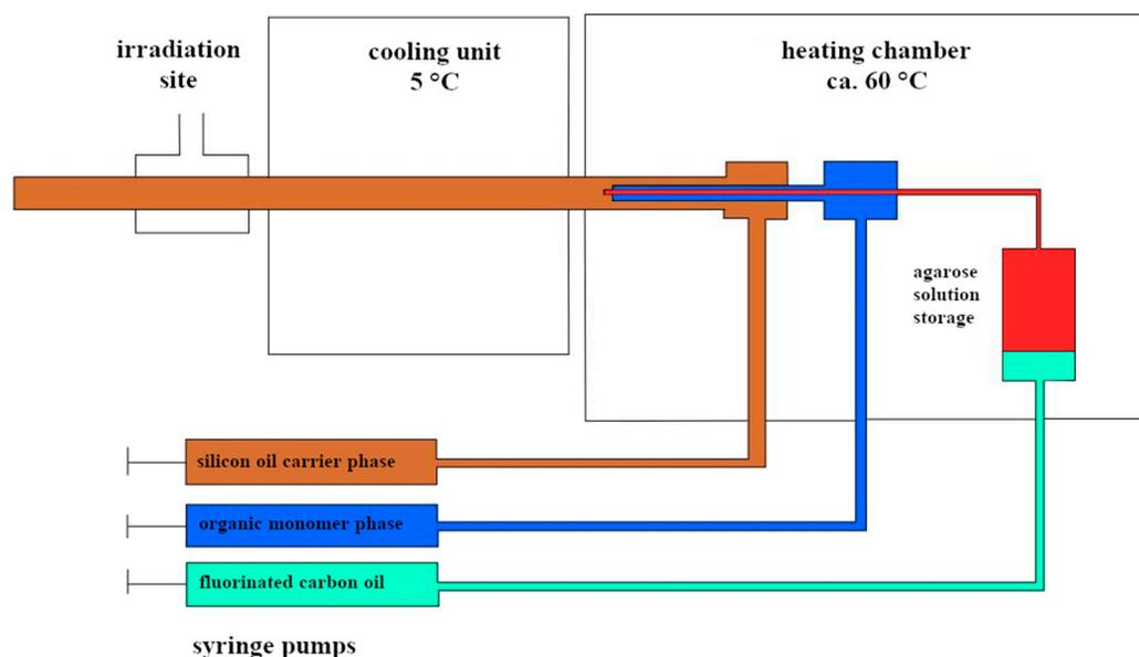
**Figure 1.** Sketch of the microfluidic device.
