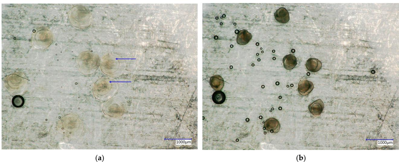
**Figure 4.** Microscopic images of composite particles with improved shells at (a) 26 °C and (b) 38 °C, respectively. NIPAM 0.85 M, AA 0.12 M, BDDA 0.076 M, and dark agarose cores; arrows indicate the voids between the core and shell.
