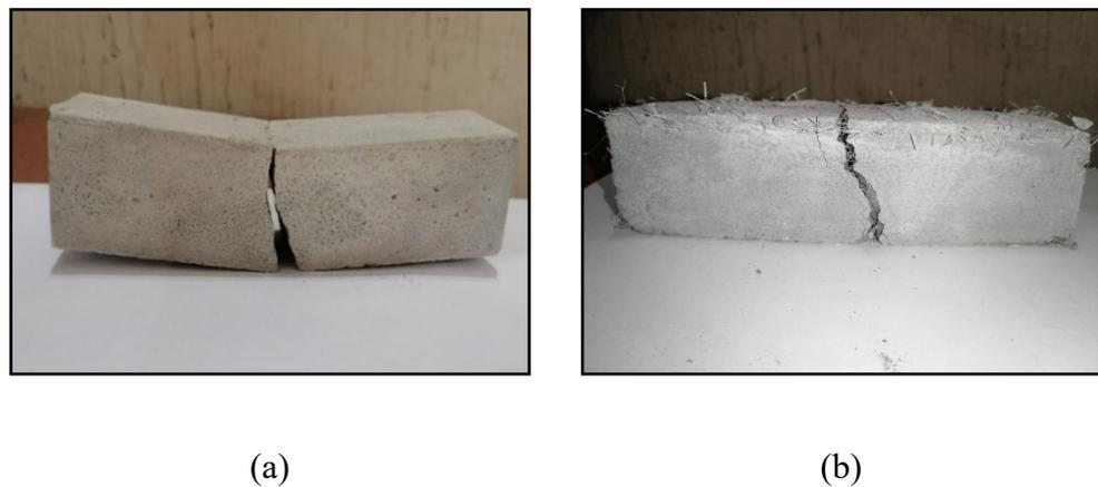
**Figure 9.** Failure modes of prisms under bending load: (a) Brittle failure in bending in C, (b) Fiber pullout failure in bending in M4.
