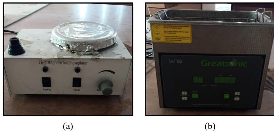
**Figure 3.** Apparatus used for sonication of CNTs: (a) Magnetic stirrer, (b) Bath sonicator.
