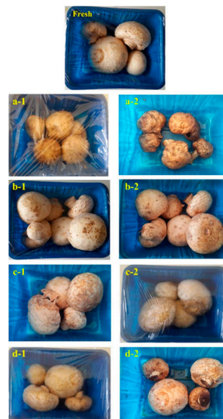
Figure 7. The physical appearance of fresh mushrooms packed with pure bacterial cellulose-based membranes (a) and active membranes containing pomegranate peel extract (b), green tea extract (c), and rosemary extract (d) after 5 days (1) and 15 days (2) of storage at 4 °C (reprinted with permission from [92]; copyright (2024) with permission from John Wiley and Sons).
