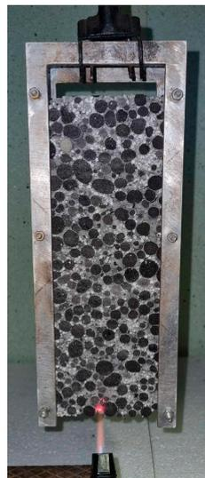
**Figure 3.** The ignitability of a vertically oriented test specimen when exposed to a small flame.
