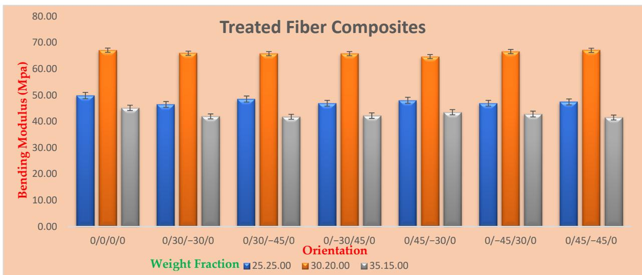
Figure 9. Flexural strength variation of natural fiber reinforced with treatment composite for different volume fractions and different orientations.
