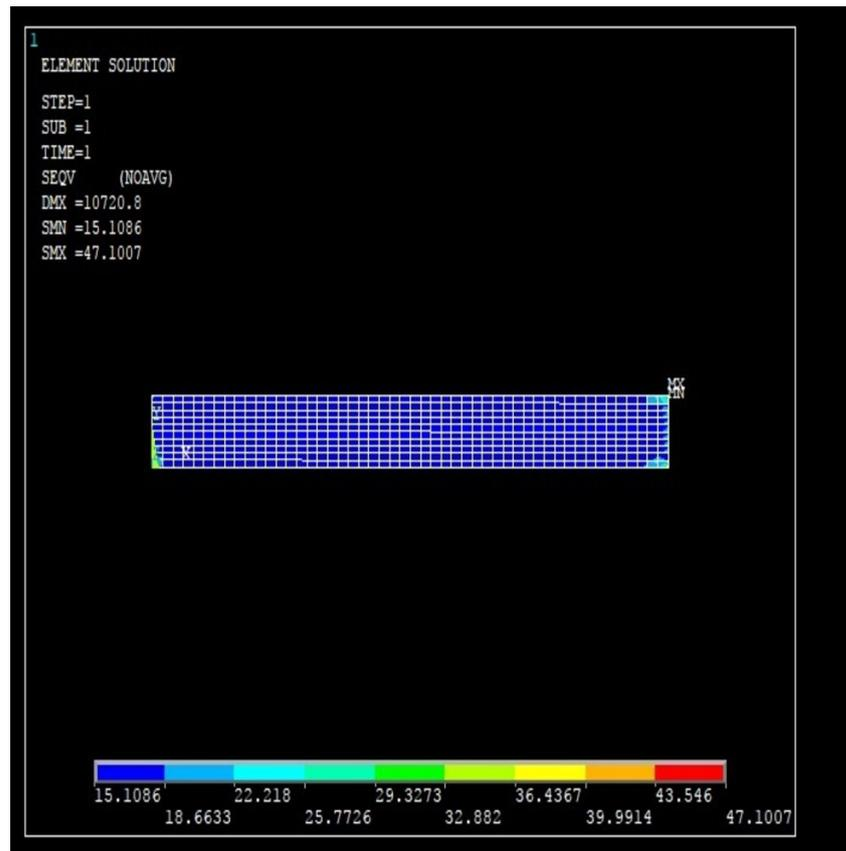
(b) simulated tensile test results for 30B/20Ba composite with 0/30/-30/0 orientation
