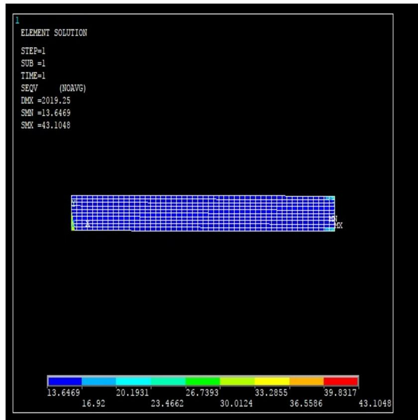
(d) simulated tensile test results for 35B/15Ba composite with 0/-30/45/0 orientation
