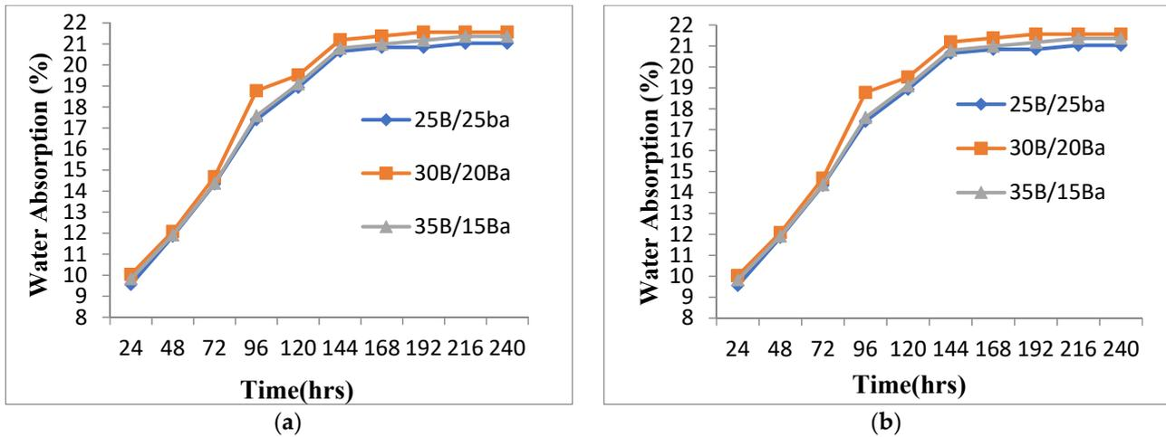
Figure 11. Water absorption curves (a) untreated banyan and banana fiber-reinforced composites and (b) treated banyan and banana fiber-reinforced composites.
