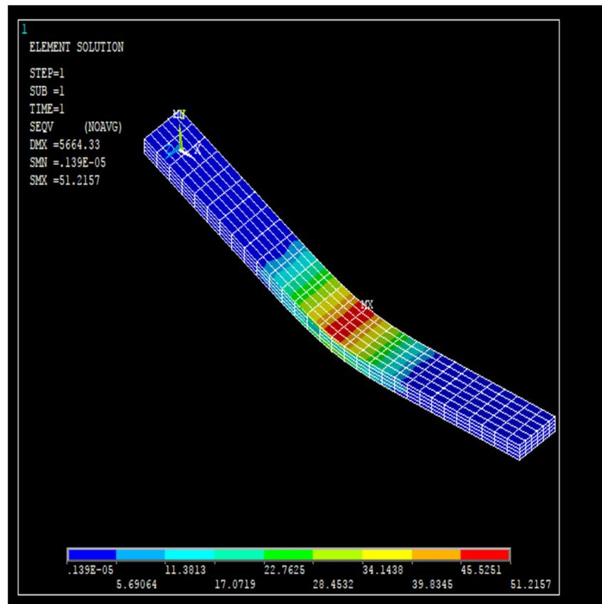
(c) simulated bending test results for 30B/20Ba composite with 0/45/-45/0 orientation
