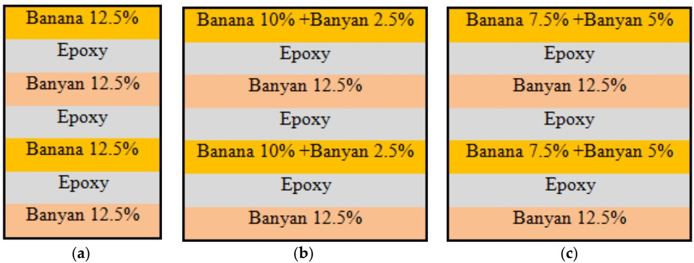
**Figure 4.** Schematic layout of the ply sequence for banyan (B) and banana (Ba) fiber epoxy hybrid composites. (a) 25B/25Ba, (b) 30B/20Ba and (c) 35B/15Ba.
