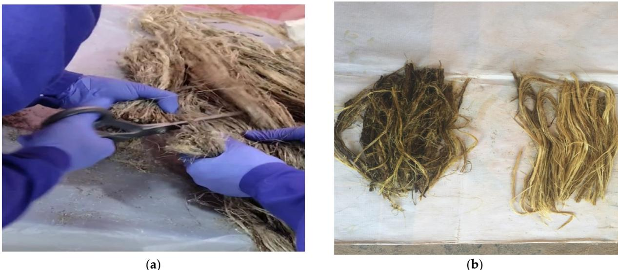
**Figure 2.** (a) Cutting of banyan and banana fibers. (b) The treated fibers of banyan and banana.
