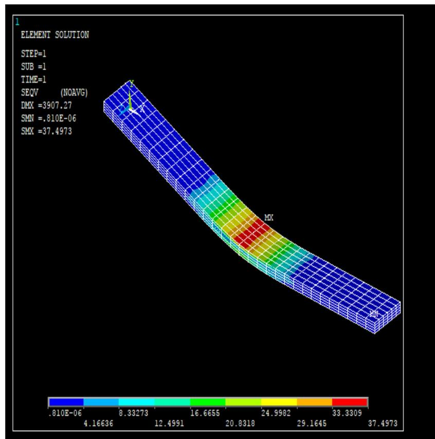
(a) simulated bending test results for 25B/25Ba composite with 0/45/−45/0 orientation
