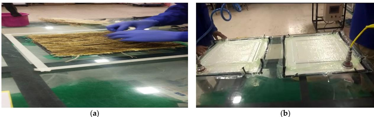
Figure 3. (a) the fibers are stagnating. (b) Vacuum bag process.
