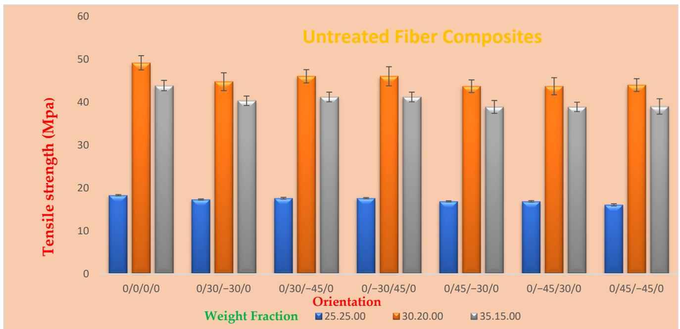
Figure 7. Tensile strength variation of natural fiber reinforced without treatment composite for different volume fractions and different orientations.
