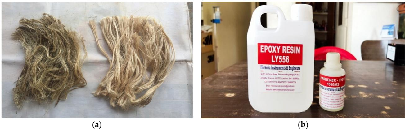
**Figure 1.** (a) raw banyan (B) and banana (Ba) fibers. (b) The hardener (HY951) and epoxy resin (LY556).
