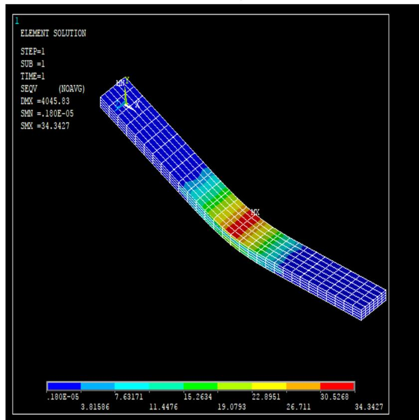
(e) simulated bending test results for 35B/15Ba composite with 0/-30/45/0 orientation
