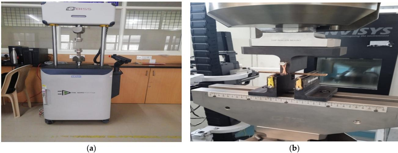
**Figure 6.** (a) A servo-hydraulic-type Nano Plug-n'-Play Series Universal testing machine. (b) Three-point bend fixture.
