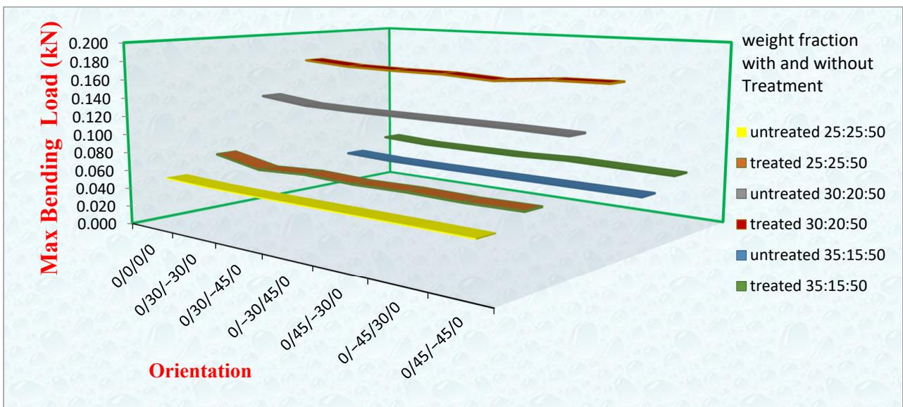
Figure 10. Bending load carrying capacity of natural fiber reinforced with and without treatment composites for different volume fractions and different orientations.
