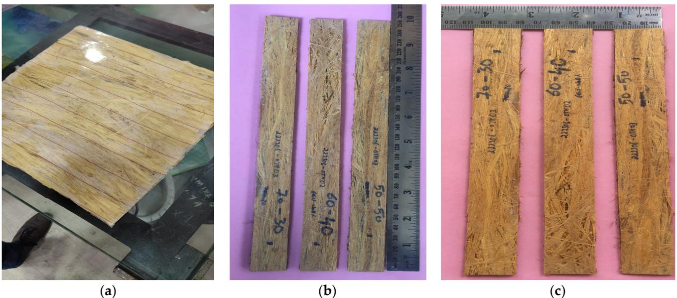
**Figure 5.** (a) Laminate composite, (b) Tensile test composite specimens 30 and (c) Bending test specimens.
