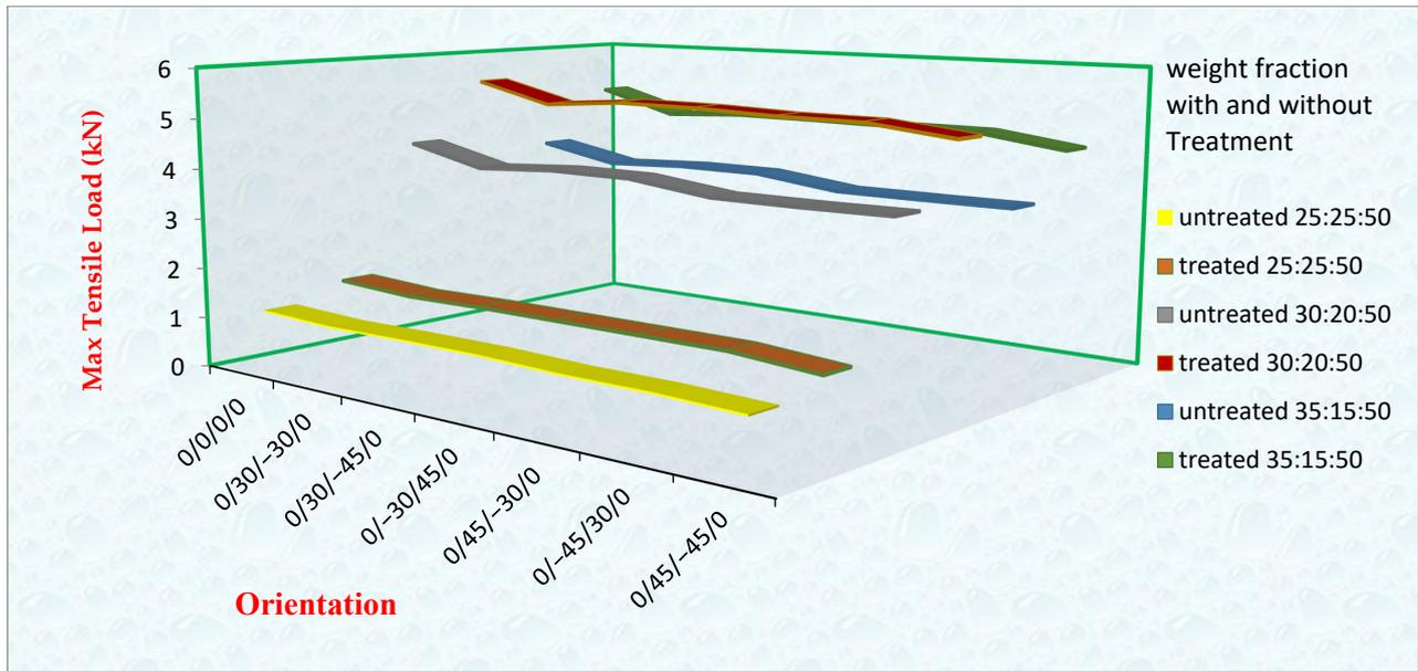
Figure 8. Tensile load carrying capacity of natural fiber reinforced with and without treatment composite for different volume fractions and different orientations.
