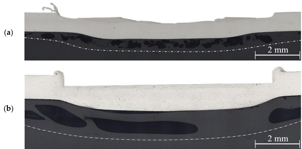
Figure 7. Cross sections of the weld conditions (a) PL_0.2_15_S and (b) PL_0.2_30_S.
