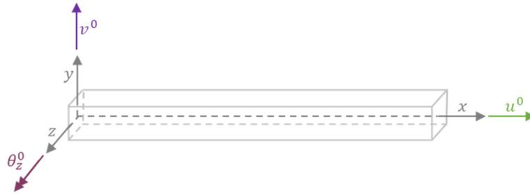
**Figure 4.** Beam representation and local coordinate system.
