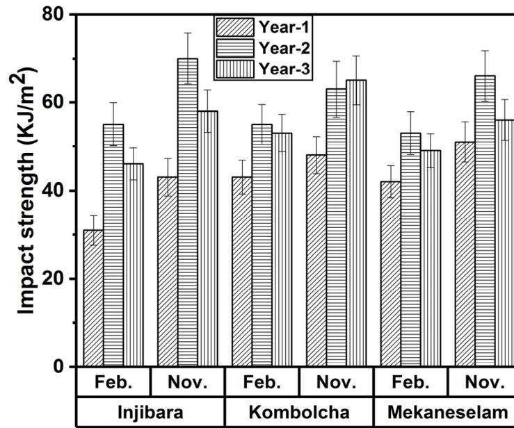
Figure 10. Impact strength of BFEPs.
