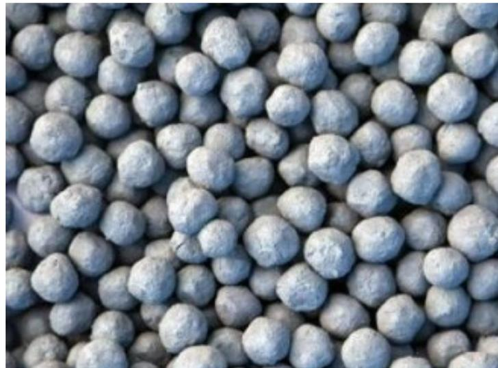
**Figure 3.** Produced composite chromite pellets.
