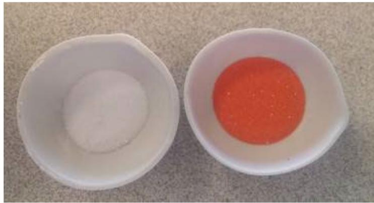
**Figure 5.** Raw materials for synthesis of chromite pigment.
