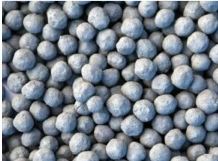
**Figure 3.** Produced composite chromite pellets.
