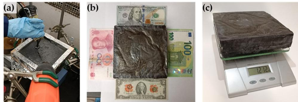
**Figure 2.** Pouring molten SunBG<sub>90</sub> into a foil-lined brick mold (a) to form the brick (b) used for ISO 8302, with a mass of 1.212 kg (c).
