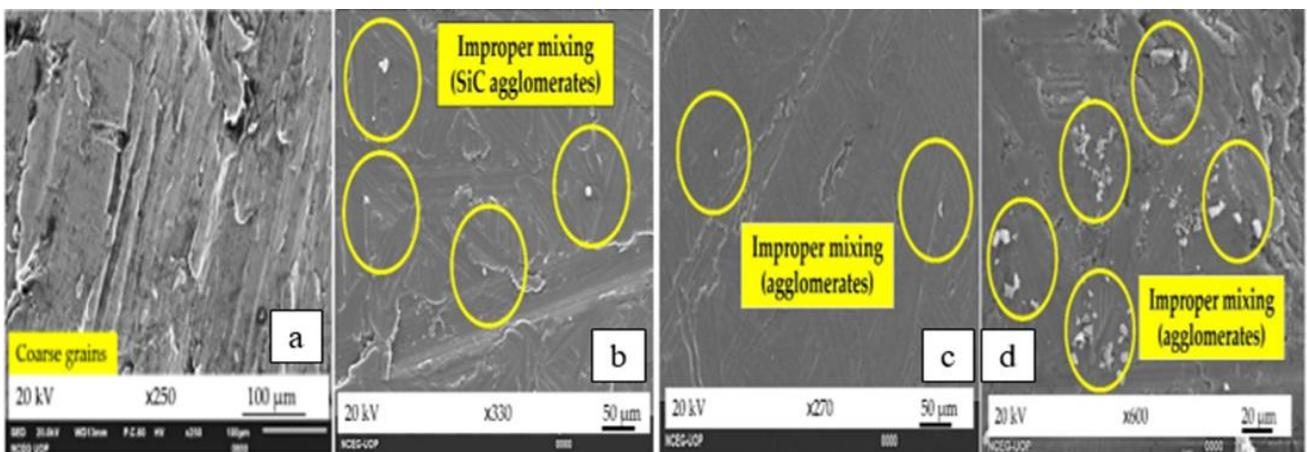
**Figure 12.** SEM image’s microstructural study of: (a) AA7075 alloy, (b) AA7075–5wt%SiC, (c) AA7075–5wt%SiC–3wt%RHA, and (d) AA7075, 5 wt% SiC, 3 wt% RHA, 1 wt% CES.
