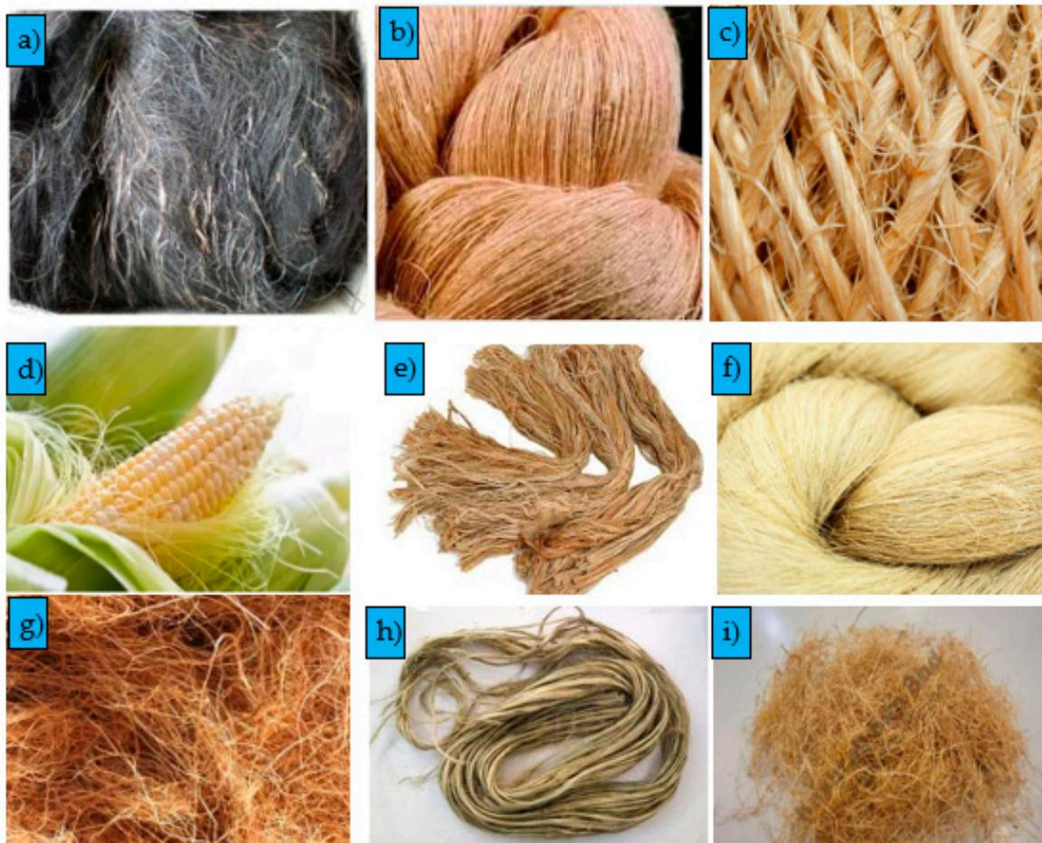
**Figure 1.** Diverse applications for hybrid natural/synthetic reinforced fiber polymer matrix. (a) Sugar palm fiber (b) Pineapple fiber (c) Hemp fiber (d) Corn fiber (e) Jute fiber (f) Flax fiber (g) Coir fiber (h) Kenaf Fiber (i) EFB fiber.
