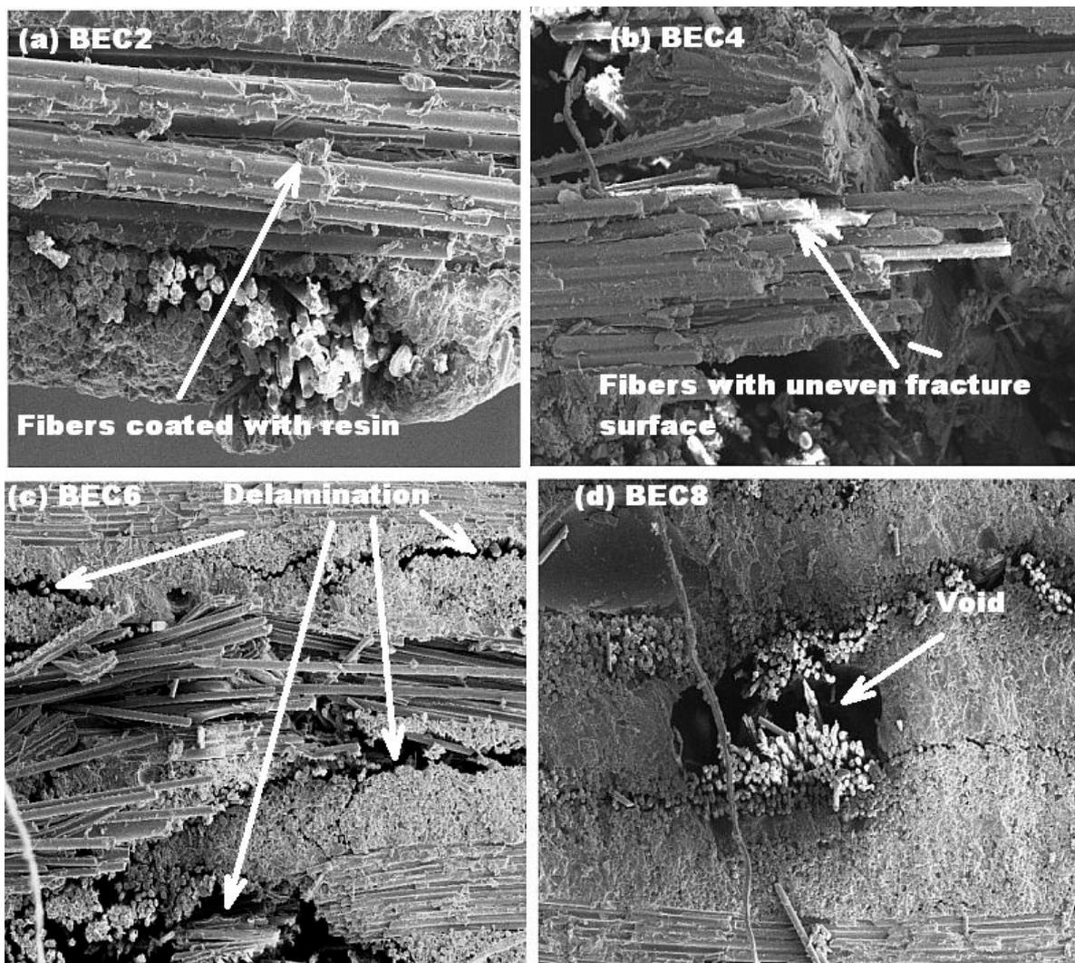
Figure 9. SEM images of fractured BEC laminates.
