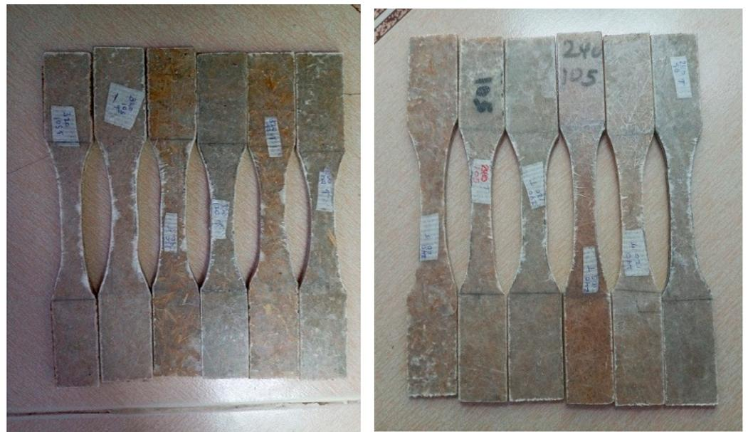
**Figure 1.** Tensile examination samples.
