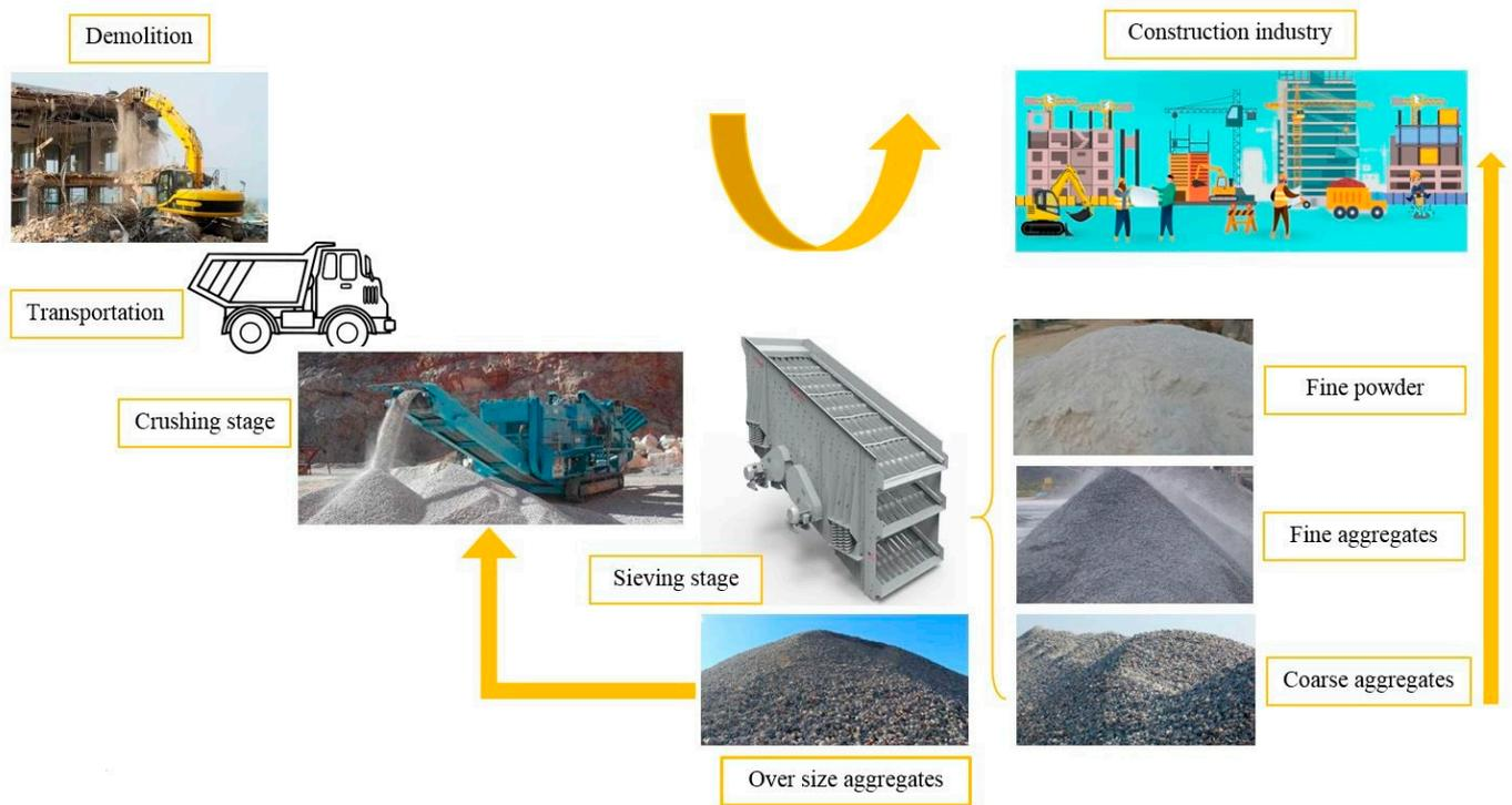
Figure 1. Recycling process of the demolished concrete.
