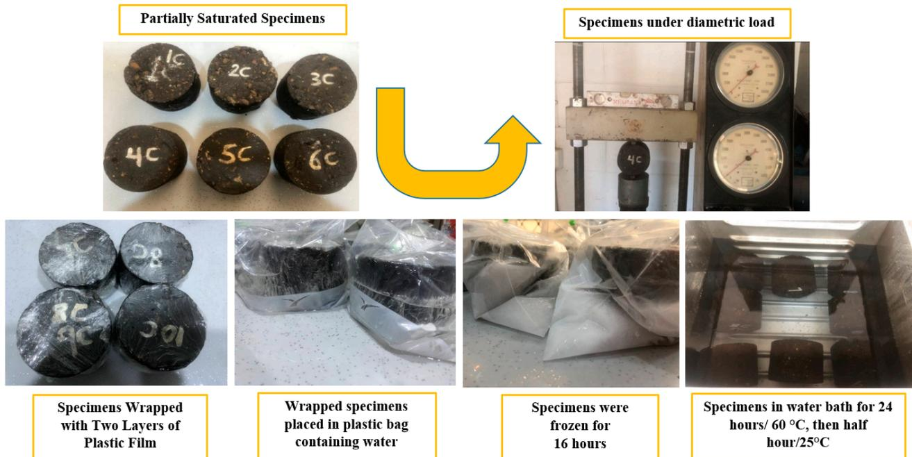
Figure 5. Specimen under ITS test.
