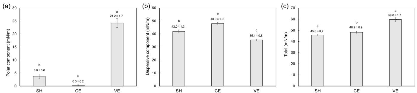
**Figure 3.** SFE of the sandblasted CAD/CAM composites, (a) polar component of SFE, (b) dispersive component of SFE, and (c) total SFE. The different alphabet letters in the figure represent statistically significant differences between the groups ( $p < 0.05$ , Tukey’s test).
