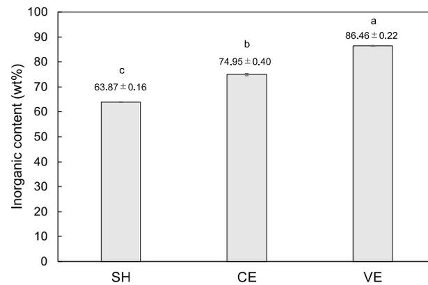
**Figure 2.** Inorganic content of the CAD/CAM composites. The different alphabet letters in the figure represent statistically significant differences between the groups ( $p < 0.05$ , Steel–Dwass test).
