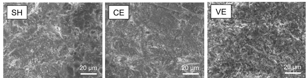
Figure 1. SEM images of the sandblasted CAD/CAM composites.
