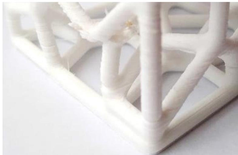
**Figure 9.** Long and thin trabeculae were susceptible to poor bonding and failure during 3D printing.
