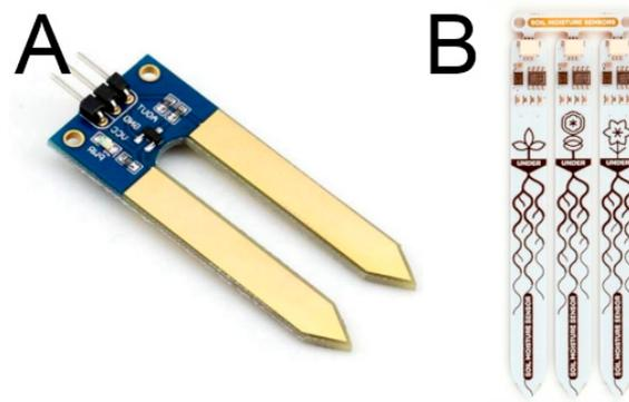
**Figure 1.** Planar soil moisture sensors based on resistance (A) and capacitance (B) measurement methodologies.
