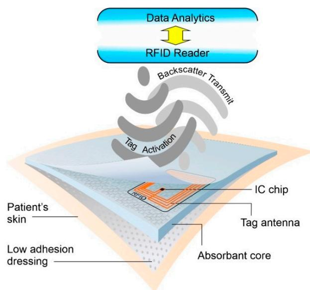
**Figure 4.** Conceptual implementation of a radio frequency identification (RFID) sensor within a wound dressing.
