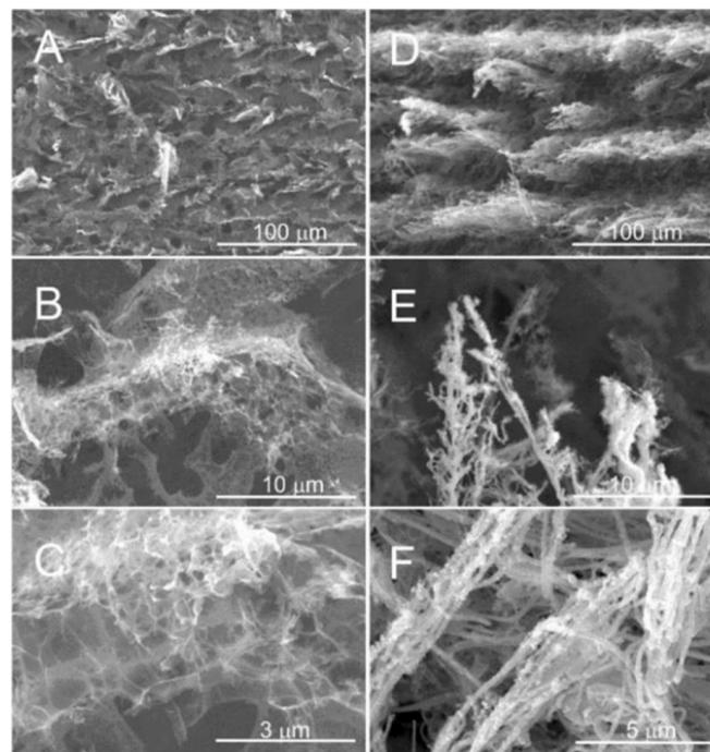
**Figure 3.** Scanning electron micrograph images of lasered polyimide tracks produced at a power of 7.5 W (A–C) and 12.5 W (D–F). Reproduced with permission [52].
