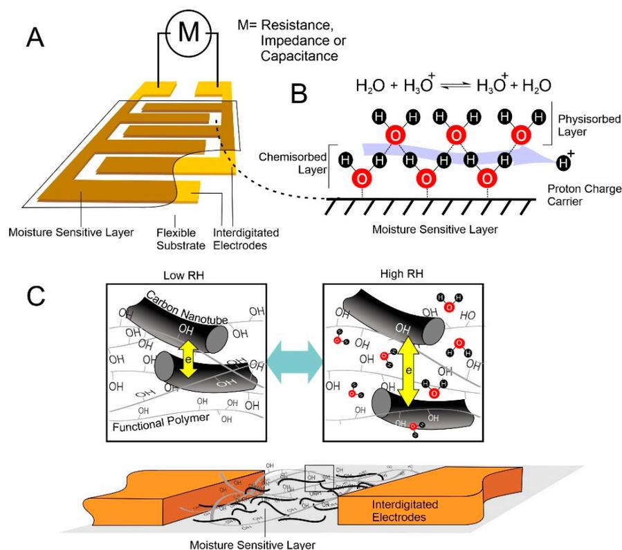
**Figure 2.** (A) Typical format of electrochemical humidity sensors and the resistive sensing methodologies associated with (B) ionic conduction and (C) physical changes brought about through swelling of the moisture sensitive film.
