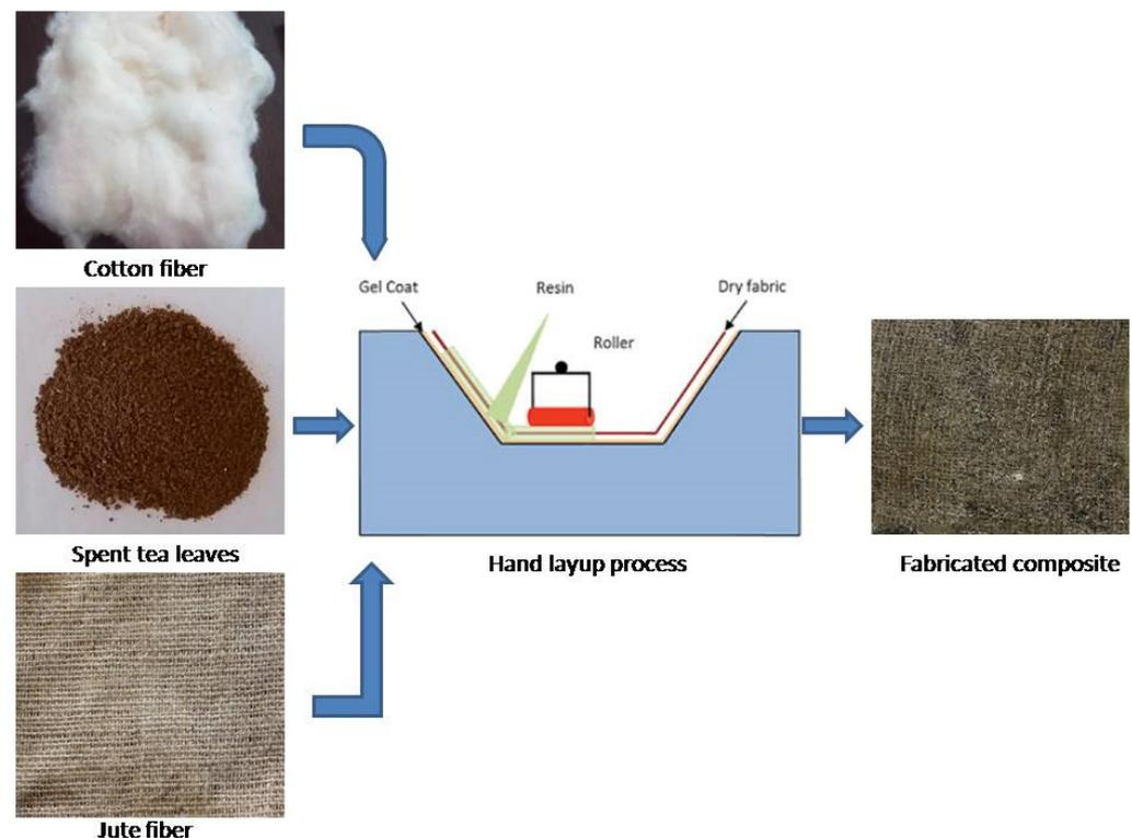
**Figure 2.** Fabrication process of the natural fibers and reinforced-particle-based composites.
