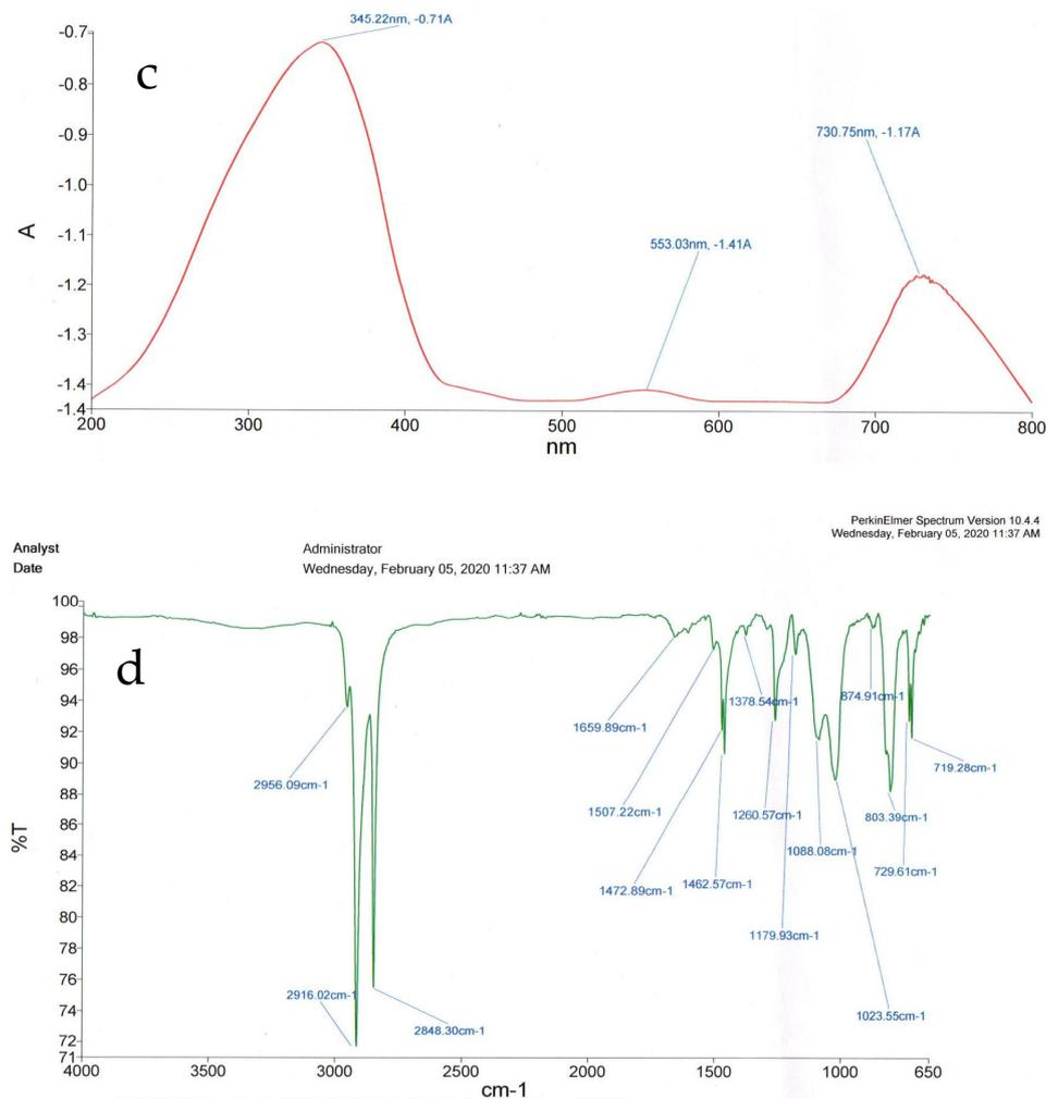
**Figure 5.** Characterization of JCJC spent tea leaf composites: (a) SEM image, (b) XRD analysis, (c) UV–Vis spectra, and (d) FTIR graph.
