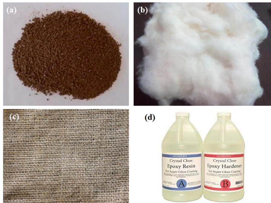
**Figure 1.** (a) Spent tea leaves, (b) cotton, (c) jute, and (d) epoxy resin and hardener.
