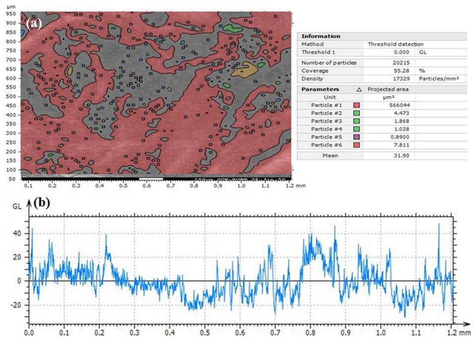
**Figure 8.** Particle analysis of JCJC spent tea leaf composites, (a) particle size detection and (b) surface profile.
