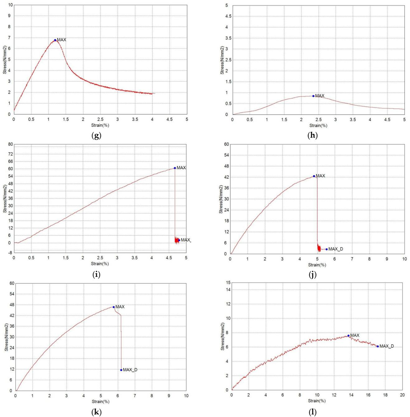
**Figure 3.** (a–d) Tensile strength graph of JCJC spent tea leaf composites: (a) S1, (b) S2, (c) S3, and (d) S4; (e–h) compression strength graph of JCJC spent tea leaf composites: (e) S1, (f) S2, (g) S3, and (h) S4; (i–l) bending strength graph of JCJC spent tea leaf composites: (i) S1, (j) S2, (k) S3, and (l) S4.
