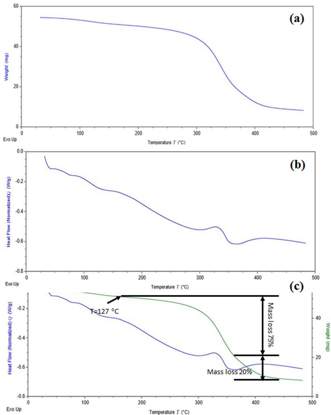
**Figure 9.** Thermal analysis of the JCJC spent tea leaf composites: (a) TGA curves, (b) DSC curves, and (c) TGA and DSC combined curves.
