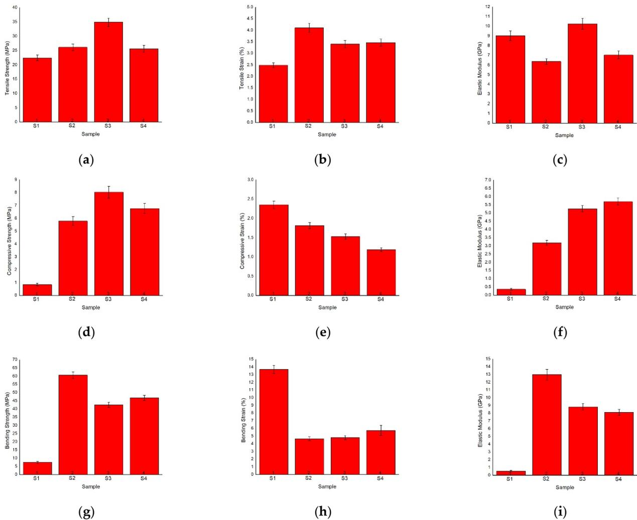
**Figure 4.** Comparison of mechanical properties in: (a) tensile strength, (b) tensile strain, (c) elastic modulus, (d) compression strength, (e) compression strain, (f) elastic modulus, (g) bending strength, (h) bending strain, and (i) elastic modulus.
