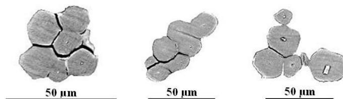
**Figure 6.** Examples of cross-sectional shape of flax technical fibres.
