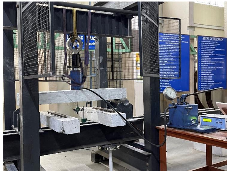
**Figure 9.** Experimental setup for testing of beam.
