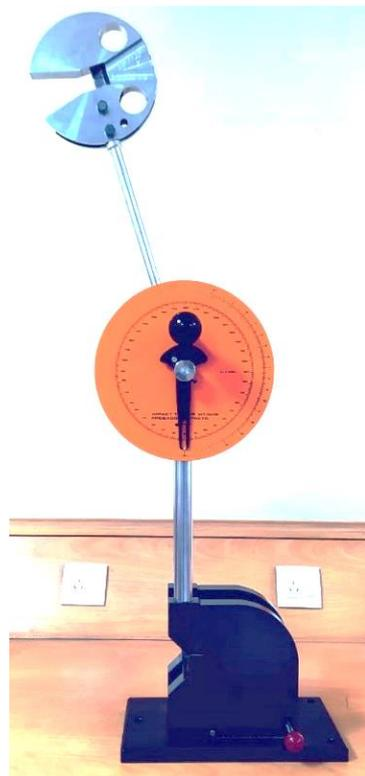
**Figure 5.** Charpy impact testing machine used for impact testing of composite samples.
