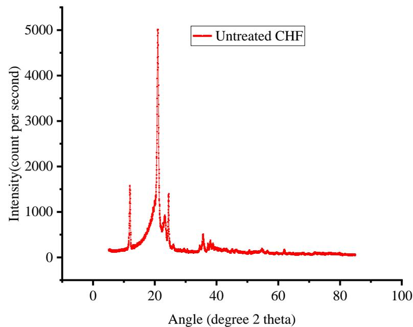
**Figure 9.** Diffraction of X-rays of untreated composites.
