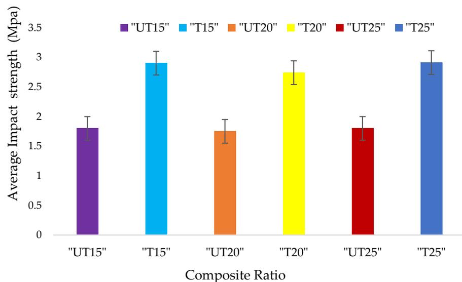
Figure 5. Impact strength test results of CH composite.
