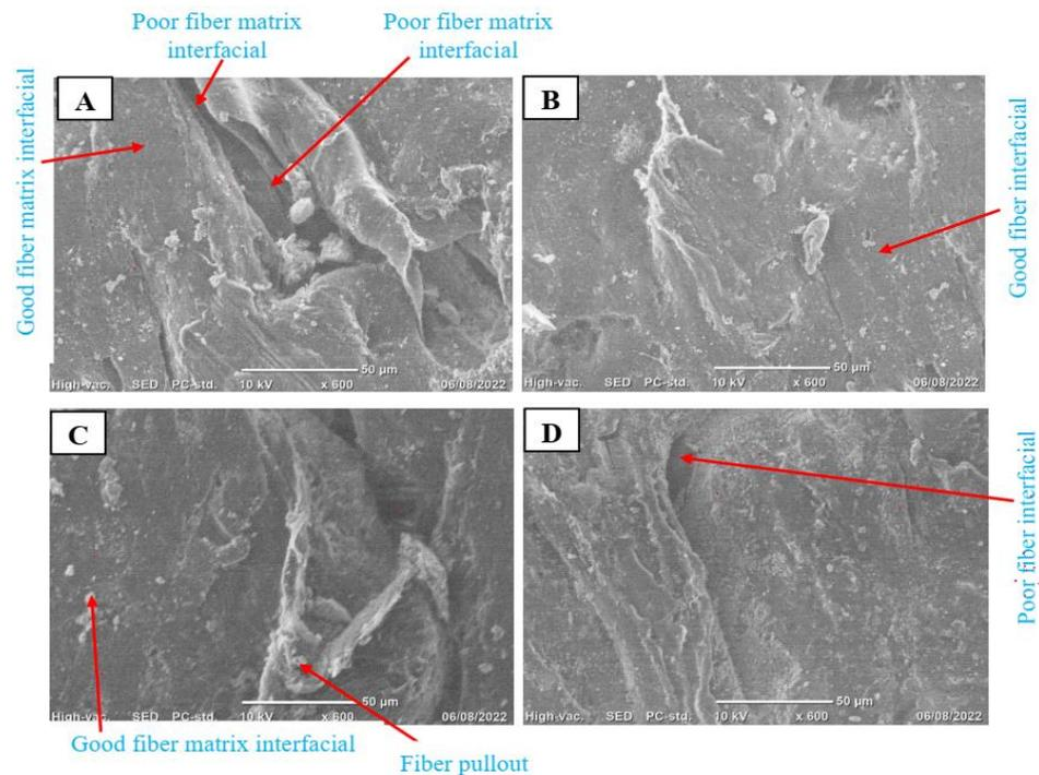
**Figure 7.** SEM image of (A) 75 wt% treated, (B) 65 wt% treated, (C) 75 wt% untreated, and (D) 65 wt% untreated CH composites.
