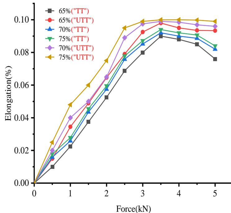
**Figure 3.** Tensile force-elongation diagram of treated and untreated CH composites. Here, 65% TT, 65% UTT, 70% UTT, 70% TT, 75% TT and 75% UTT represent 65% of treated CH, 65% of untreated CH, 70% of untreated CH, 70% of treated CH, 75% of untreated CH and 75% of treated CH in the composite mixtures, respectively.
