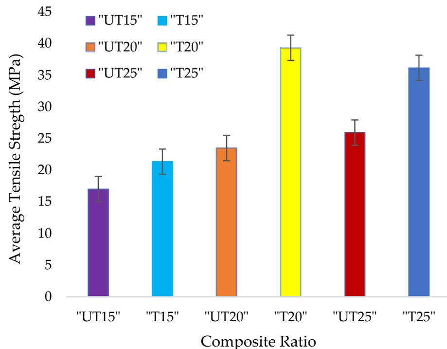
**Figure 2.** Tensile strength test results. UT15, UT20, UT25, T15, T20, and T25 represent 15% of untreated CH, 20% of untreated CH, 25% of untreated CH, 15% of treated CH, 20% of untreated CH and 25% of untreated CH in the composite mixtures, respectively.
