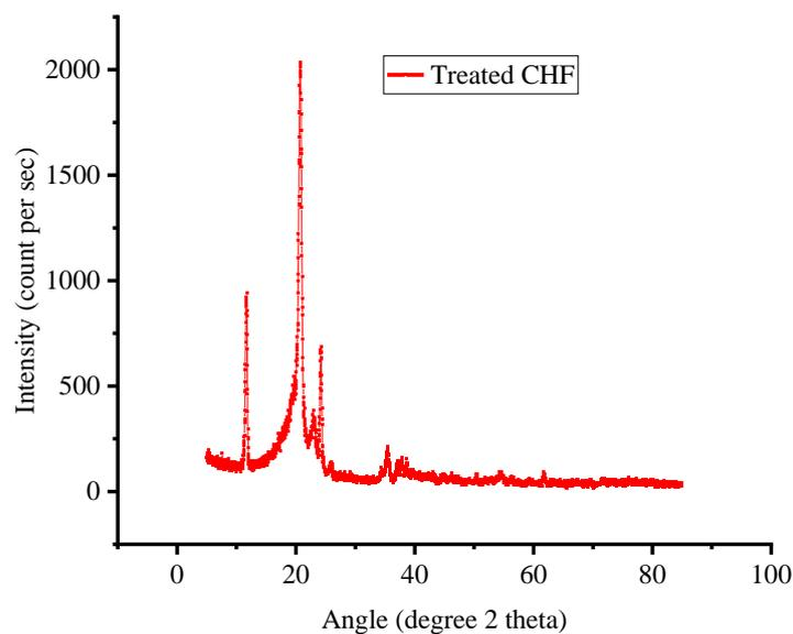
**Figure 8.** Diffraction of X-rays of NaOH-treated composites.
