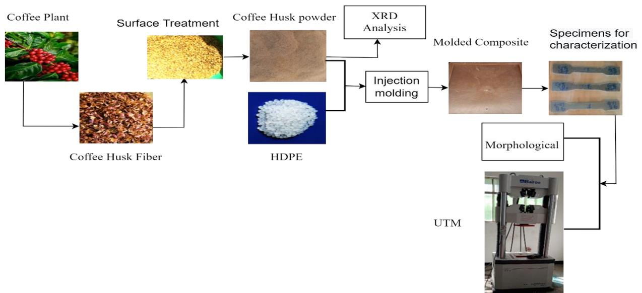
**Figure 1.** Representation of the processing sequence to produce UC and TC composites with their characterization.
