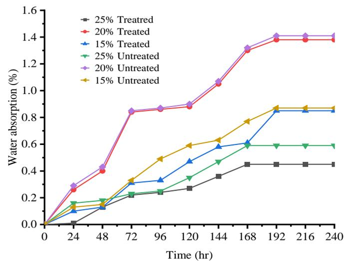
**Figure 6.** Moisture absorption test results of CH composites.
