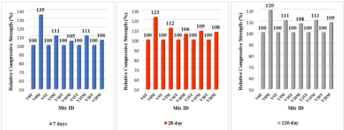
Figure 11. Effect of MW on compressive strength of volcanic concrete at 7, 28, and 120 days.
