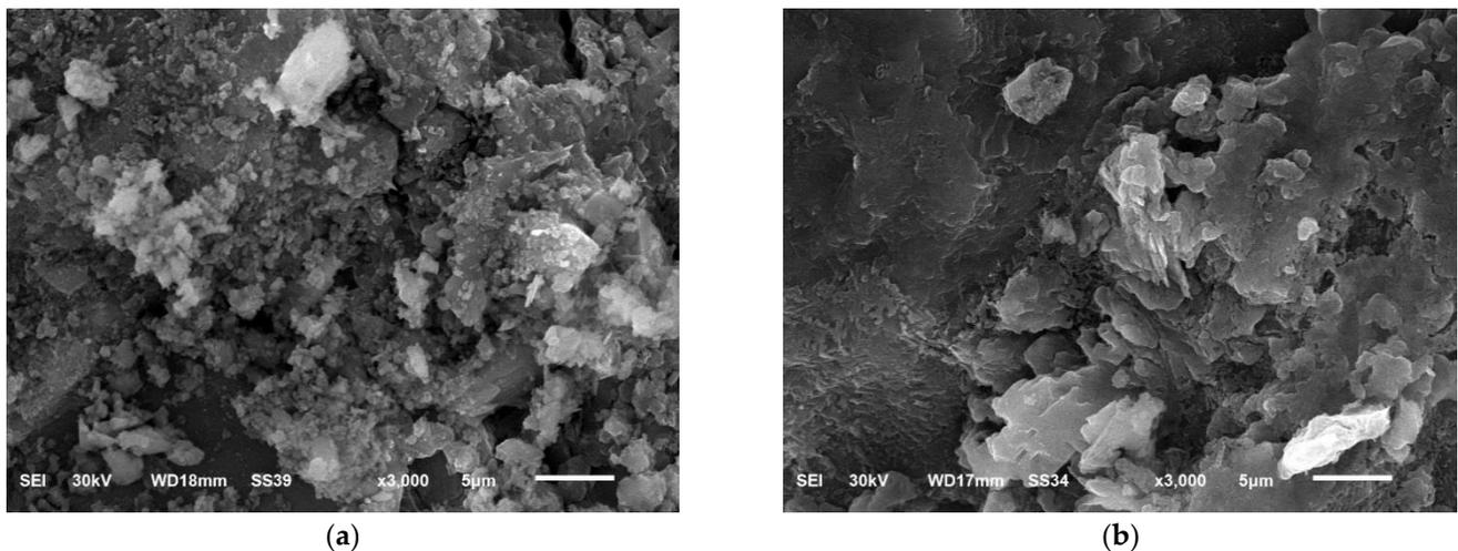
Figure 12. SEM images of the fracture surface of volcanic concrete made with MW: (a) 0%VA and (b) 5% VA.
