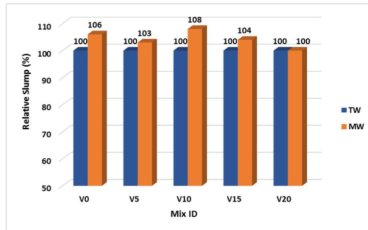
Figure 8. Effect of magnetized water on volcanic concrete slump.
