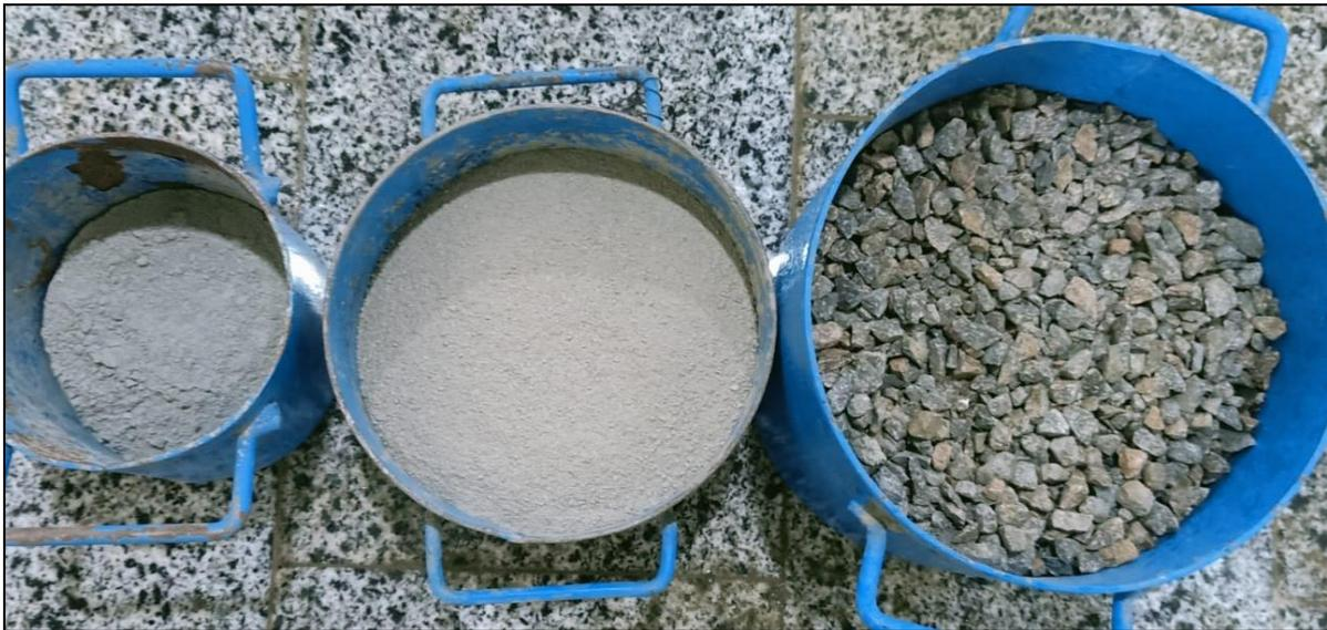
**Figure 2.** Volcanic rocks as coarse aggregate, fine aggregate, and volcanic ash.
