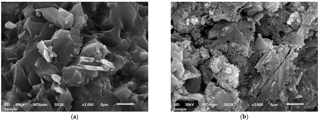
Figure 10. SEM images of the fracture surface of volcanic concrete made with TW: (a) 0%VA and (b) 5% VA.
