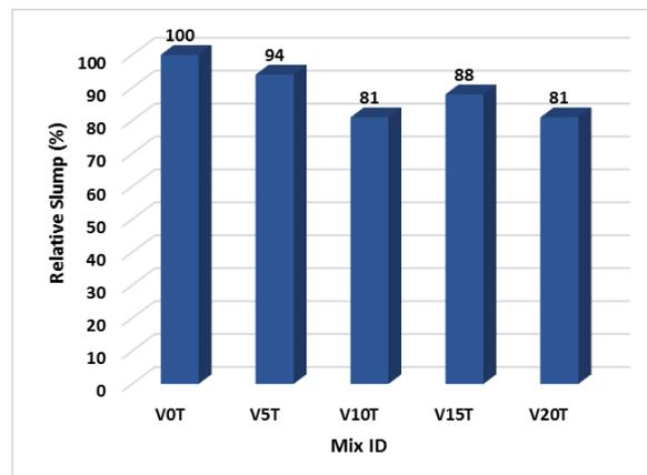
**Figure 7.** Effect of VA ratio on the slump of volcanic concrete made with tap water.
