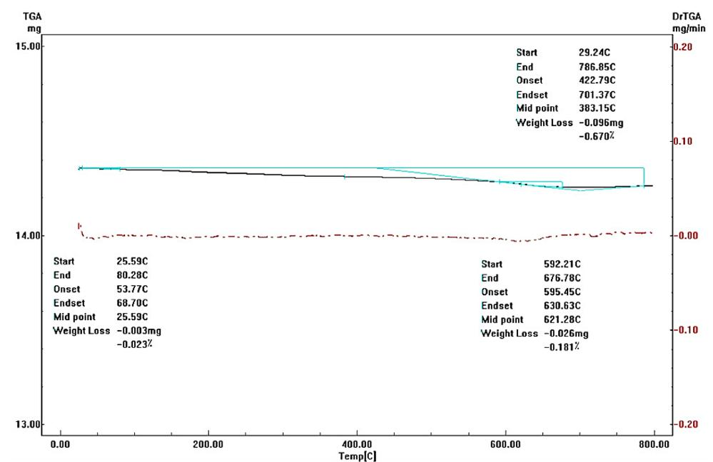
**Figure 4.** TGA analysis of VA.
