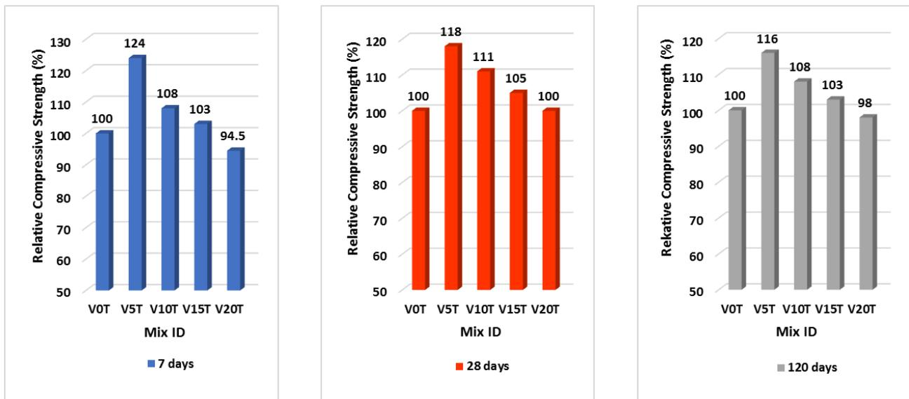
Figure 9. Effect of different ratios of VA on volcanic concrete compressive strength mixed with tap water.
