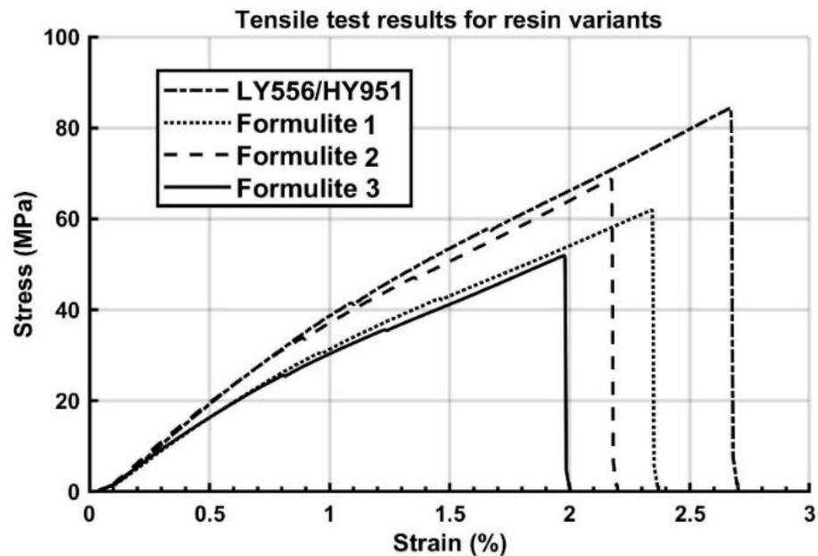
Figure 8. Stress–strain graph for samples tested for tensile properties.
