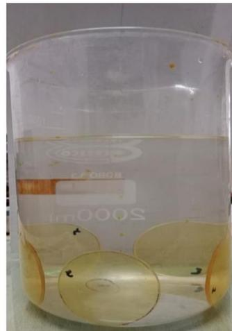
**Figure 7.** Water absorption specimens immersed in a container of distilled water.
