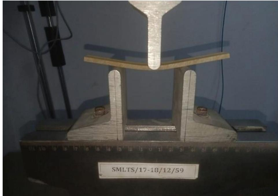
**Figure 4.** Equipment setup for flexural test specimen in a computerized universal testing machine from DAK system incorporation.
