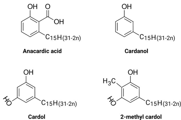
**Figure 1.** Chemical structure of CNSL with its components.
