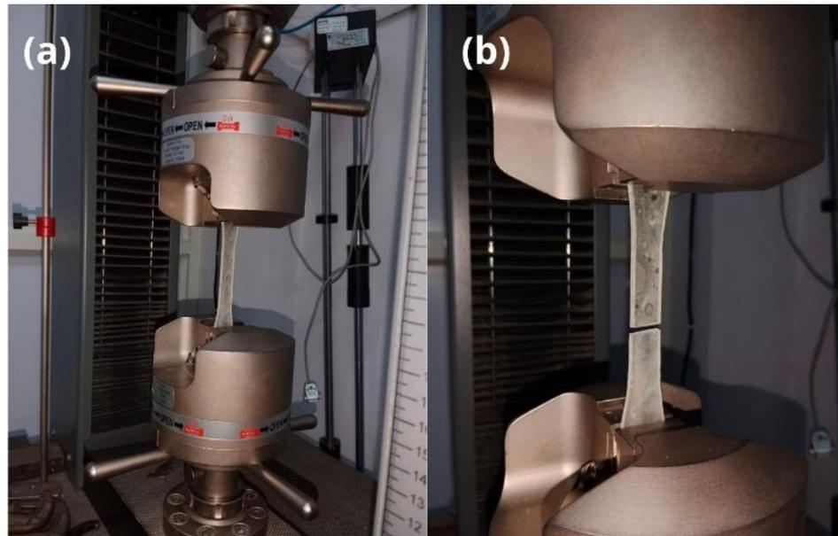
**Figure 3.** Equipment setup for tensile test specimen in a computerized universal testing machine from DAK system incorporation, (a) tensile specimen in a fixture, (b) fractured tensile specimen.
