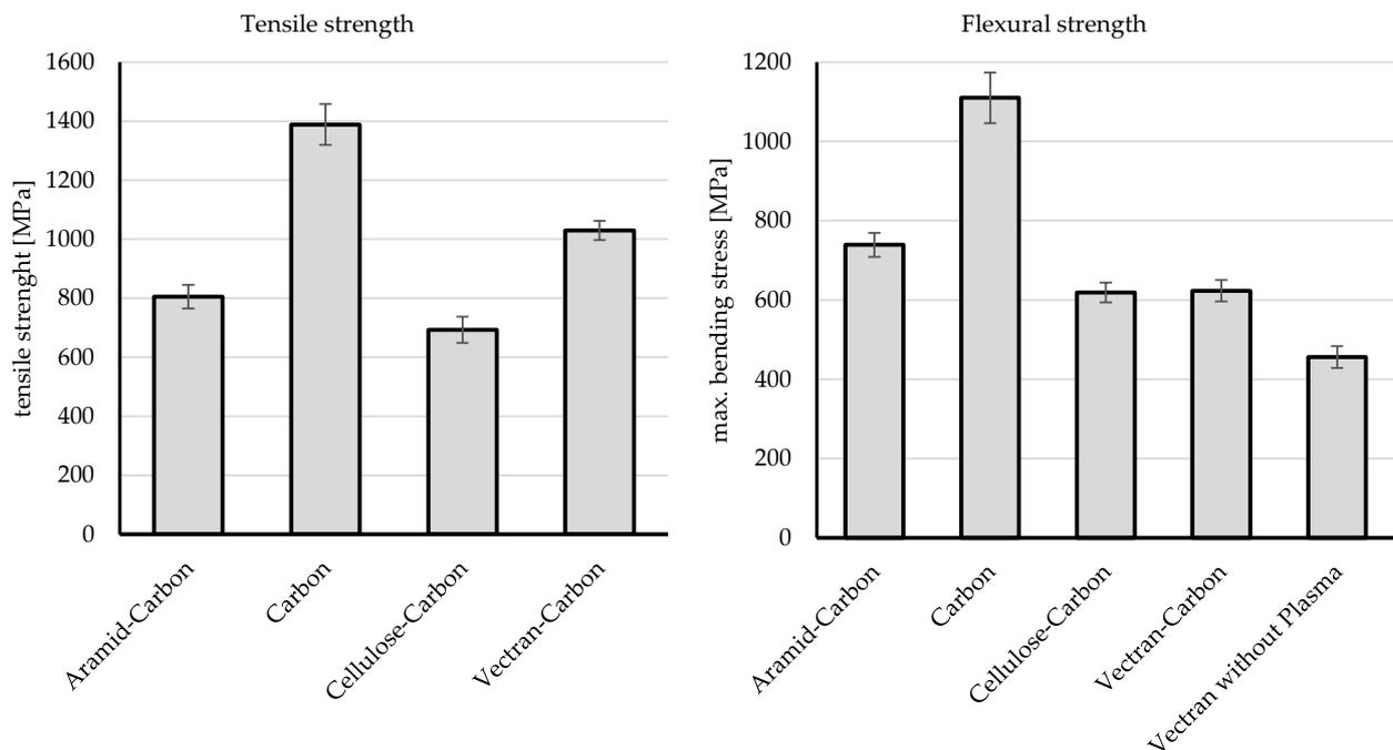
**Figure 5.** Strength in tensile and flexural direction.
