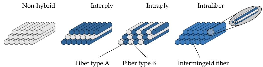
**Figure 1.** Hybridization types of composites in comparison.
