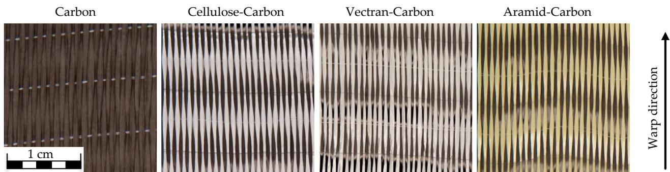
**Figure 3.** Hybrid and non-hybrid UD-fabrics produced.
