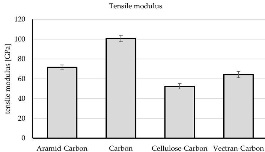
**Figure 8.** Tensile modulus in fiber direction.
