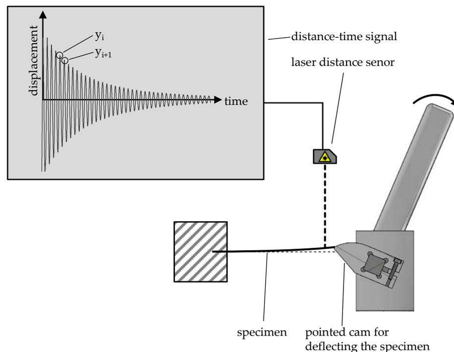
**Figure 4.** Apparatus for measuring material damping.
