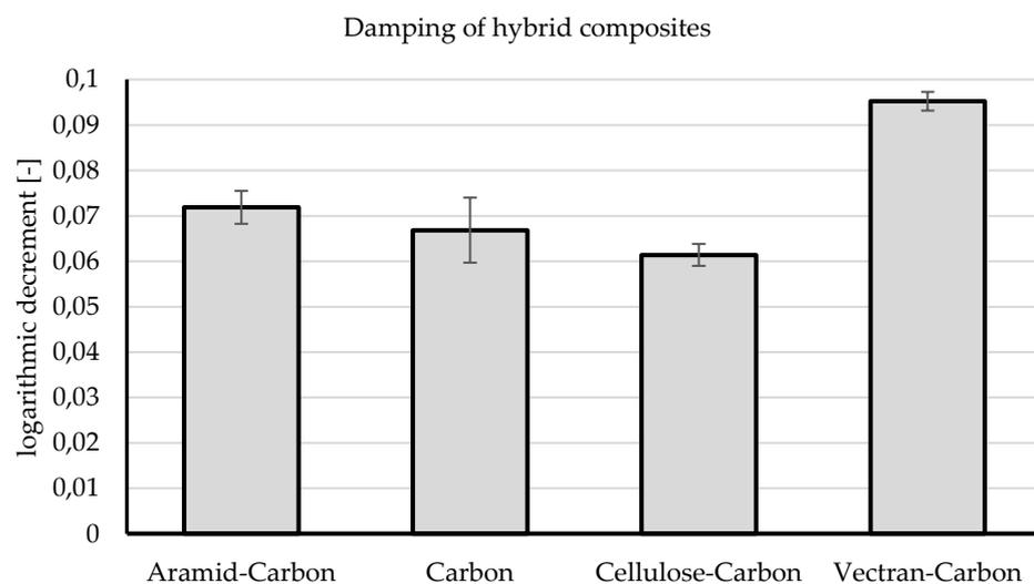
**Figure 9.** Logarithmic decrement with the same spring stiffness.
