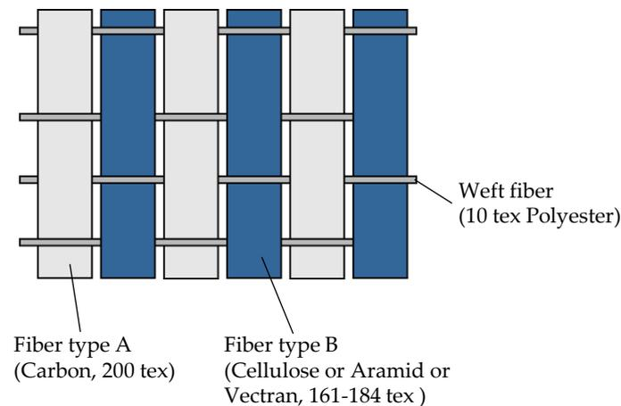
**Figure 2.** Construction of unidirectional hybrid textiles.
