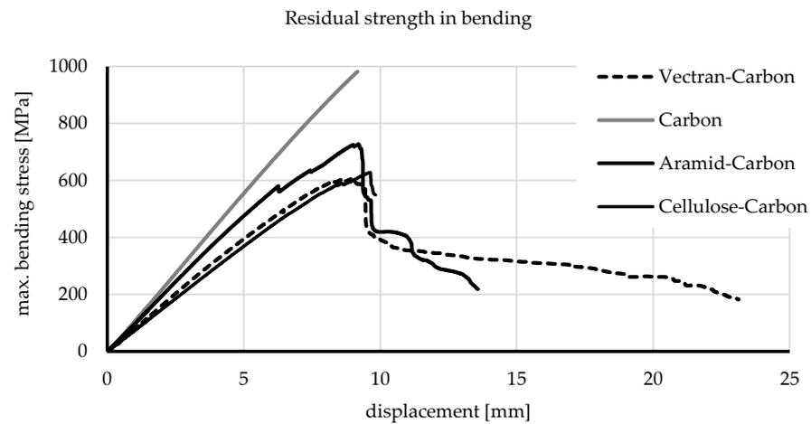
Figure 6. Fracture behavior under flexural loading.
