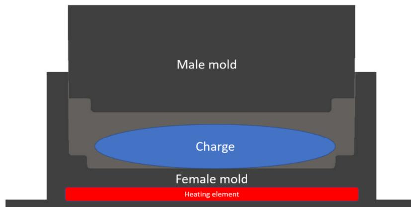
**Figure 13.** Proposed heating element for the new tooling system.
