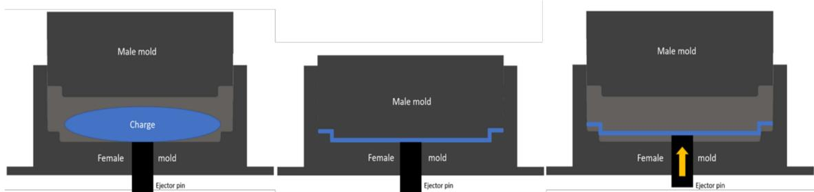
**Figure 12.** Proposed ejector pin for the new tooling system.
