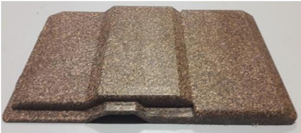
**Figure 9.** A specimen of wood fiber composite cut into shape for the compressive strength test.
