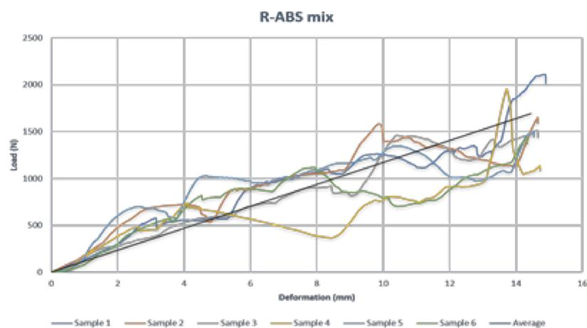
Figure 14. Compression testing results of the R-ABS mix blend.
