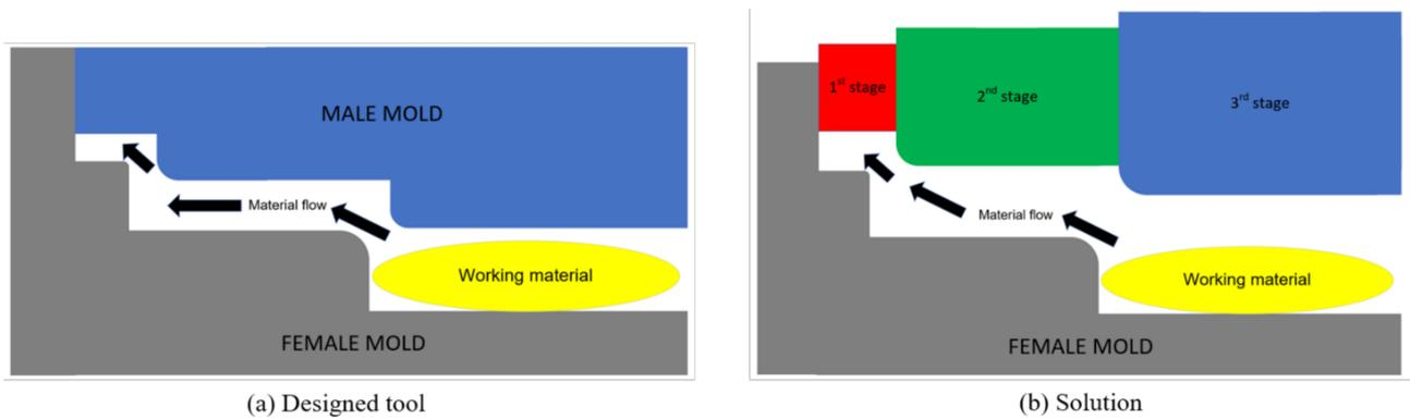
Figure 11. Illustration of (a) the designed tool for the production of the new automotive part and (b) the suggested change in the tooling system.
