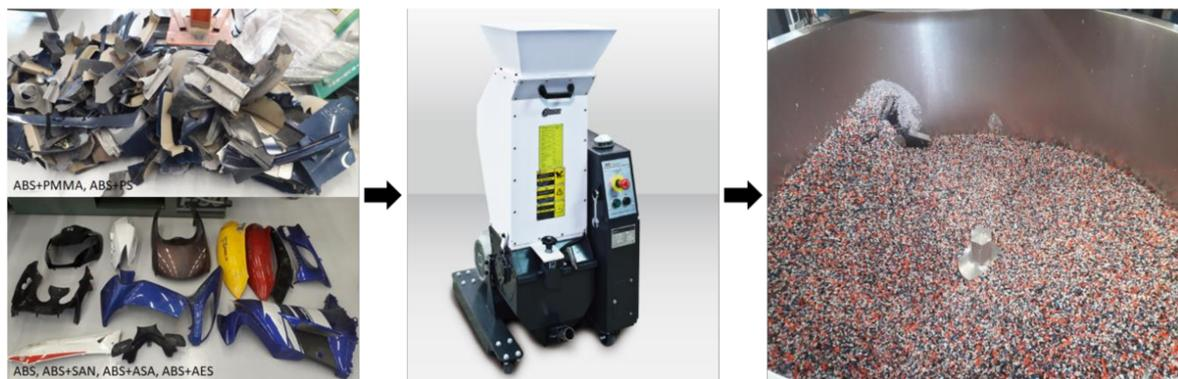
**Figure 7.** Illustration of the crushing process for the waste automotive components.
