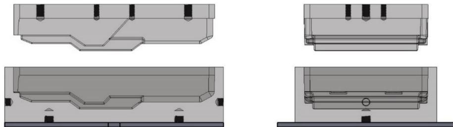
**Figure 6.** Representation of the compression molding tool in Solidworks.
