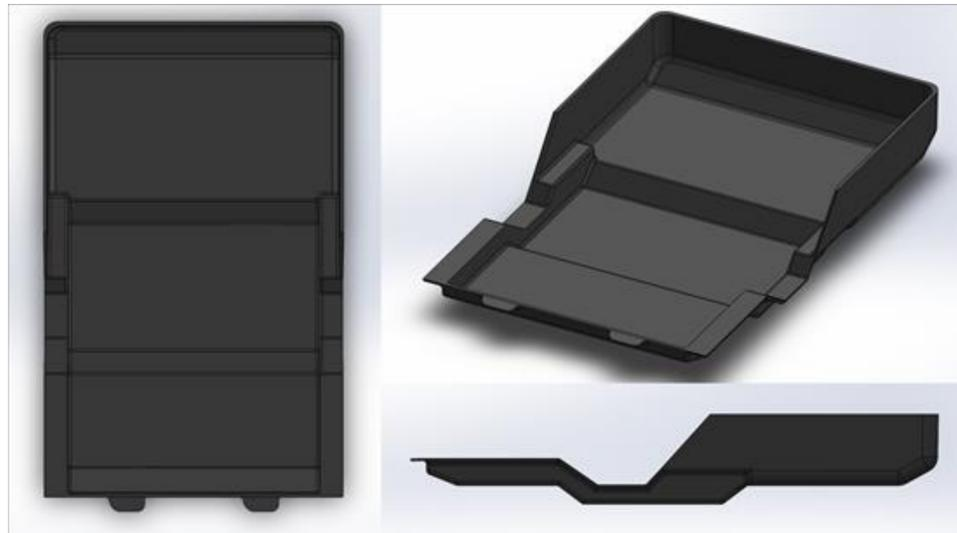
**Figure 4.** New automotive part design for the natural fiber polymer composite (NFPC) application.
