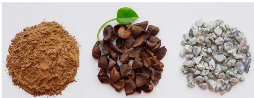
**Figure 4.** FA, OPS lightweight aggregate and crushed granite used for concrete mixtures.
