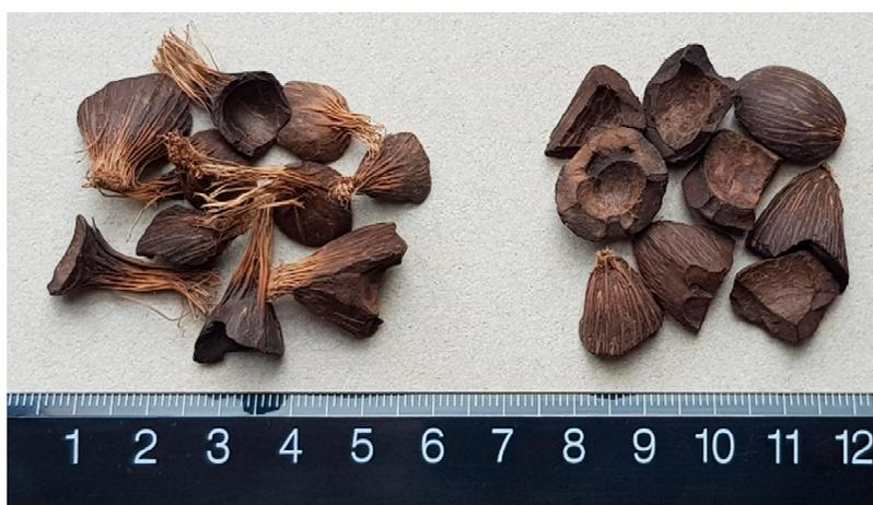
**Figure 3.** OPS aggregates before and after removing of the surface fibers.
