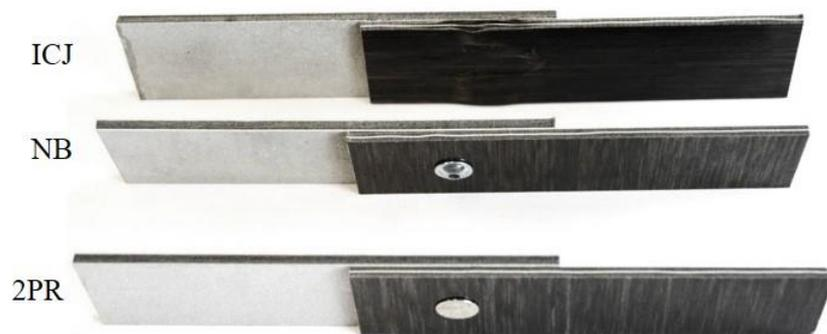
Figure 4. Joining samples of Type I and Type II for the three joining methods. NB: nut and bolt; 2PR: two-piece hollow riveting.
