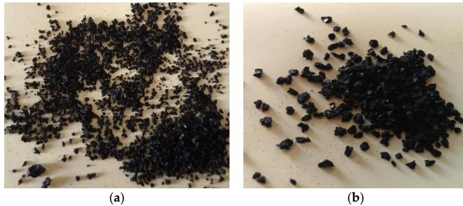
**Figure 1.** Ground tire rubber (GTR) aggregates used in this research: rubber powder (a) and rubber granules (b).
