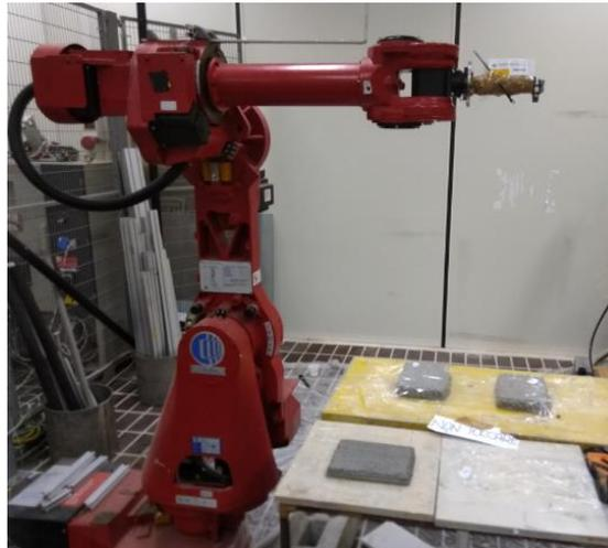
**Figure 2.** Three-axis robotic arm-based printing device.
