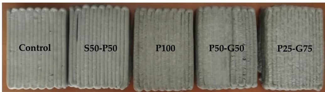
Figure 3. Hardened 3D printed slabs resulting from printability tests.
