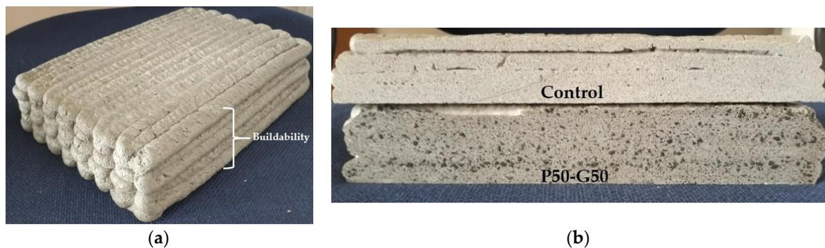
**Figure 7.** Proper buildability in the P50-G50 sample (a) and visual inspection of inter-layer adhesion in the control and P50-G50 mixes (b).
