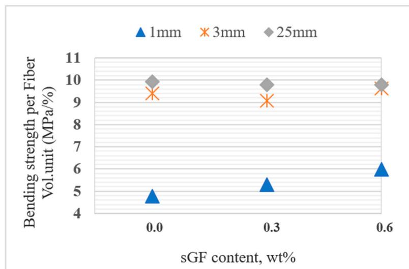
**Figure 7.** The bending strength of composites with respect to carbon fiber (CF) length and sGF addition content.
