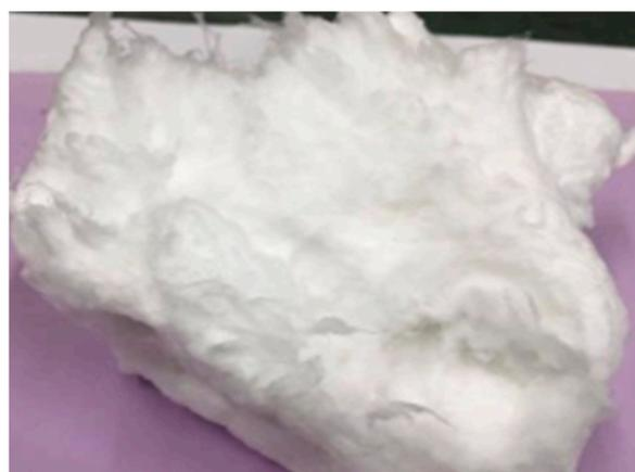
**Figure 4.** Image of original sGF before mixing with resin.
