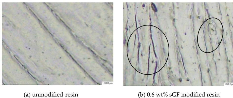
**Figure 20.** The laser microscope images of unmodified and modified resin specimens after compact tension test, showing the deflection of micro-cracks [25].
