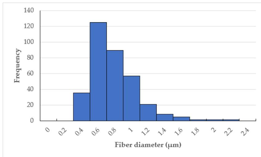
(a) The fiber diameter distribution of submicron glass fiber addition (sGF).
