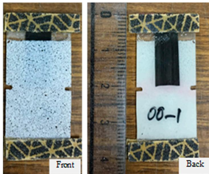
**Figure 2.** Image of model specimen with the speckle pattern from black and white paint for measuring strain distribution.
