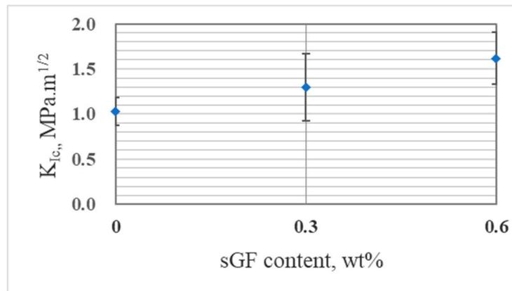
**Figure 8.** The improvement of fracture toughness of resin with the addition of sGF [25].
