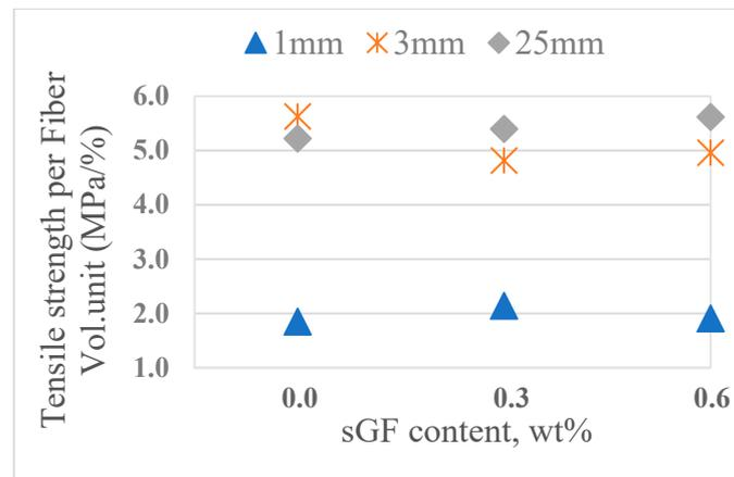
Figure 13. The tensile strength of composites with respect to CF length and added sGF content.
