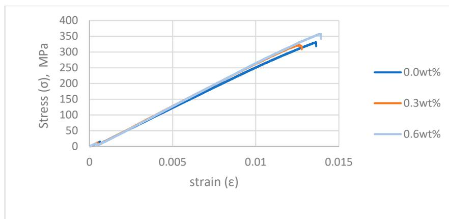
**Figure 10.** The representative stress–strain curves of 3 mm composites.
