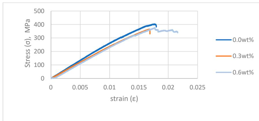
Figure 11. The representative stress-strain curves of 25 mm composites.
