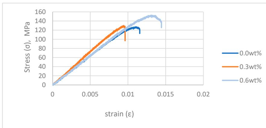
**Figure 9.** The representative stress–strain curves of 1 mm composites.
