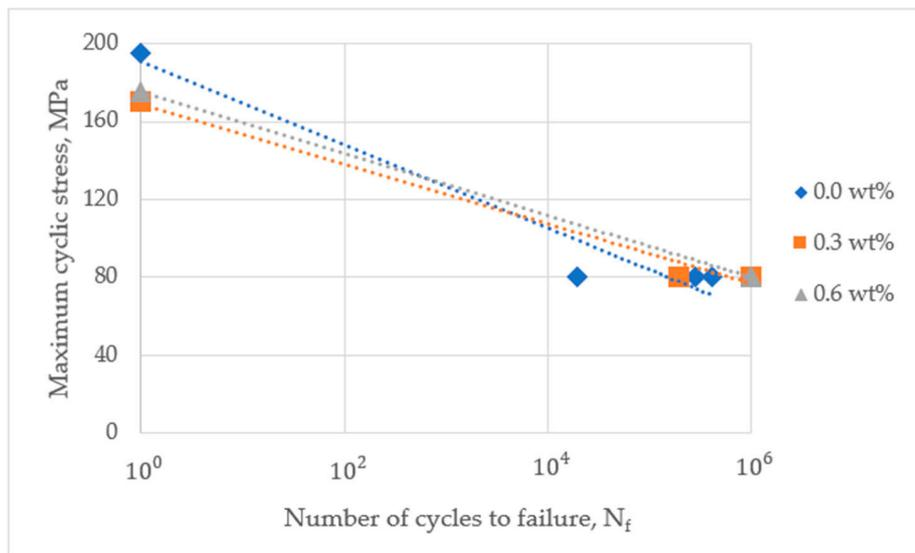
**Figure 18.** The number of cycles to failure of composite reinforced by 3 mm carbon fiber length under cyclic loading.
