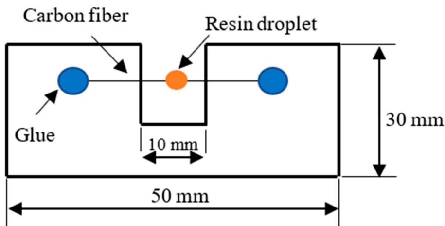
**Figure 1.** The geometry of the single carbon fiber containing one resin drop adhered to the paper frame.
