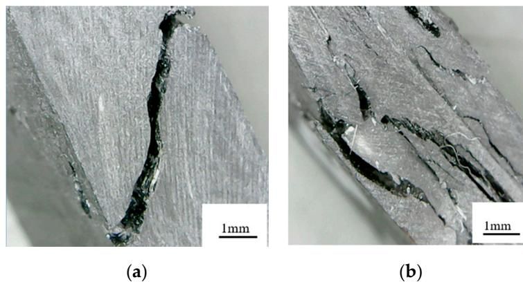
**Figure 15.** Edge fracture state of (a) 1 mm composite, (b) 25 mm composite.
