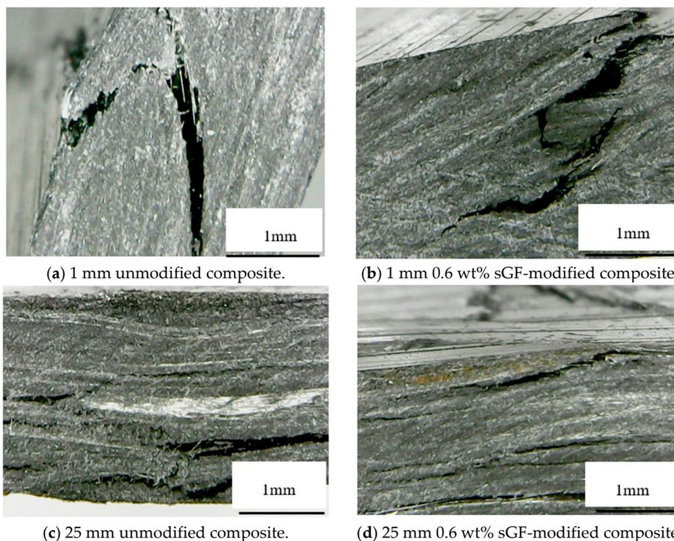
Figure 12. Fracture on the edges of composites unmodified and modified with 0.6 wt% of sGF after bending test.
