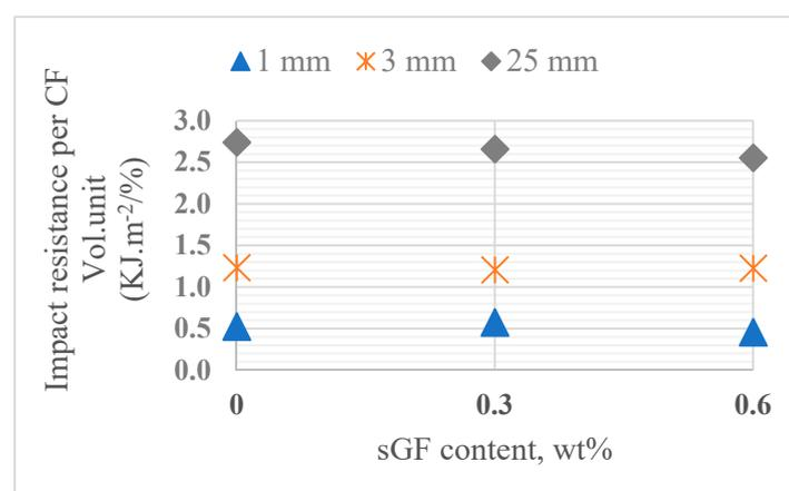
Figure 14. Izod impact resistance of composites.
