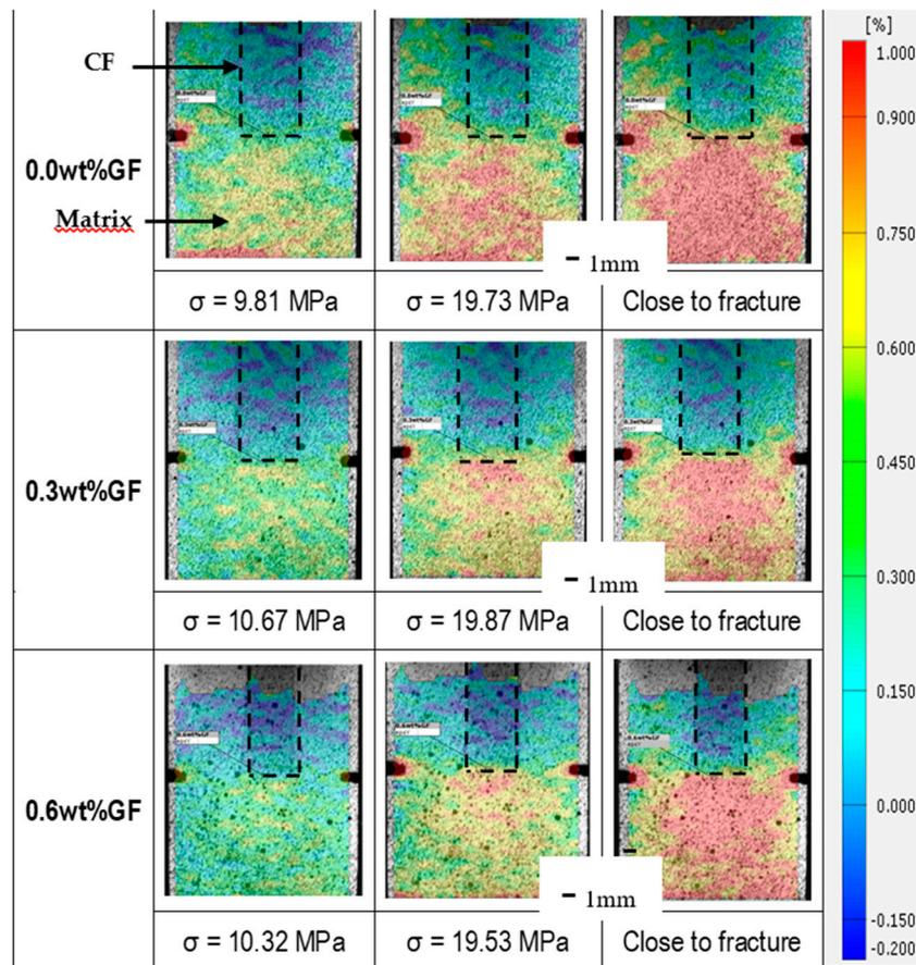
**Figure 16.** Strain distribution of composite models consisting of a single fiber bundle and unmodified/modified vinyl ester (VE).
