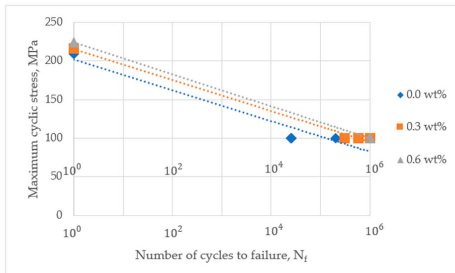
**Figure 19.** The number of cycles to failure of composite reinforced by 25 mm carbon fiber length under cyclic loading.
