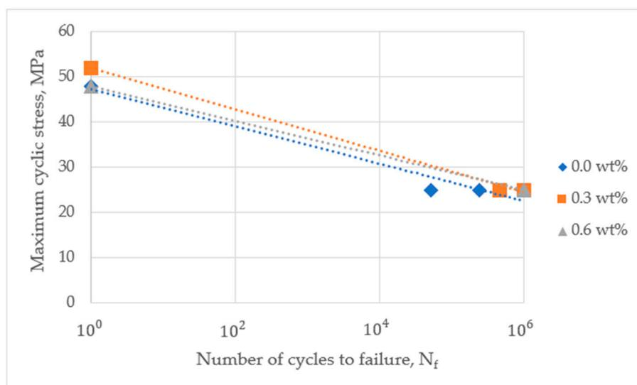
**Figure 17.** The number of cycles to failure of composite reinforced by 1 mm carbon fiber length under cyclic loading.
