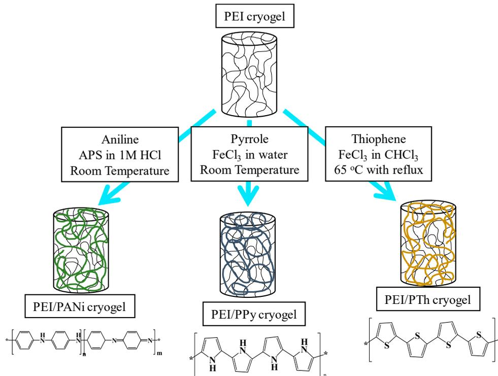
**Figure S1.** The schematic presentation of in situ synthesis of conductive PANi, PPy, and PTh polymers within PEI cryogels.
