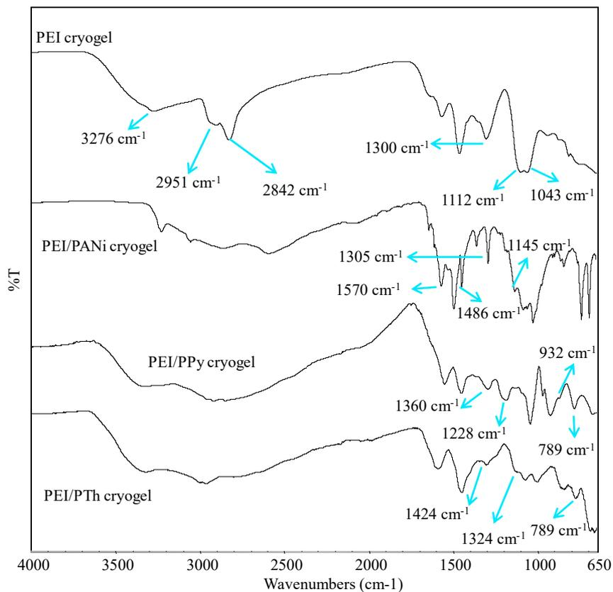
**Figure S2.** FT-IR spectra of bare PEI cryogel, PEI/PANi, PEI/PPy, and PEI/PTh cryogel composites.
