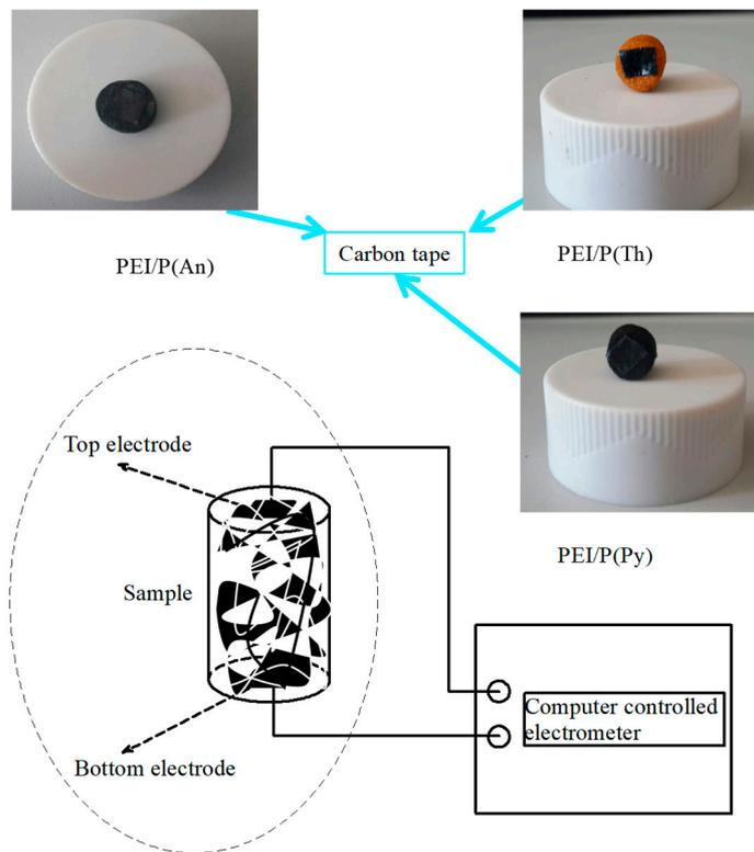
**Figure S3.** Digital camera images of PEI/PANi, PEI/PPy, and PEI/PTh cryogel composites and the schematic presentation of experimental setup used in electrical conductivity measurements.
