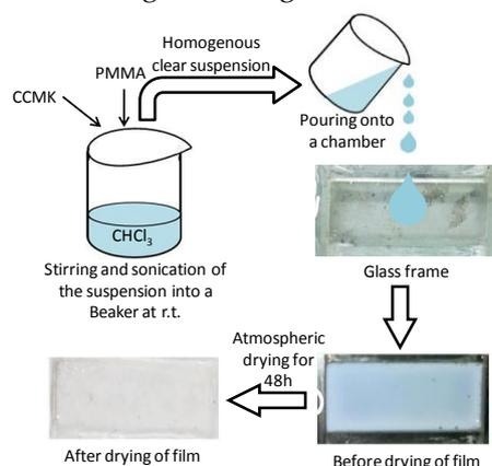
Figure S1. Illustration of fabrication technique of nanocomposite films.
