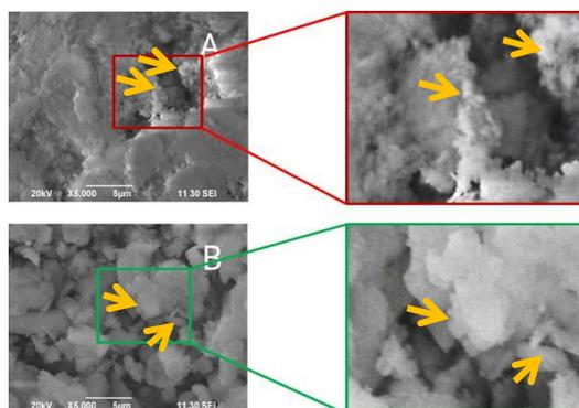
Figure S6. Electron microscope (SEM) images of kaolinite (A), modified kaolinite (B), respectively.
