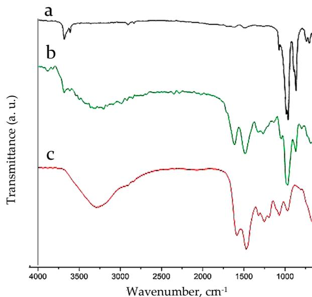
**Figure S3.** spectra of kaolinite (a), choline chloride modified kaolinite nanocomposites (b), and choline chloride (c).
