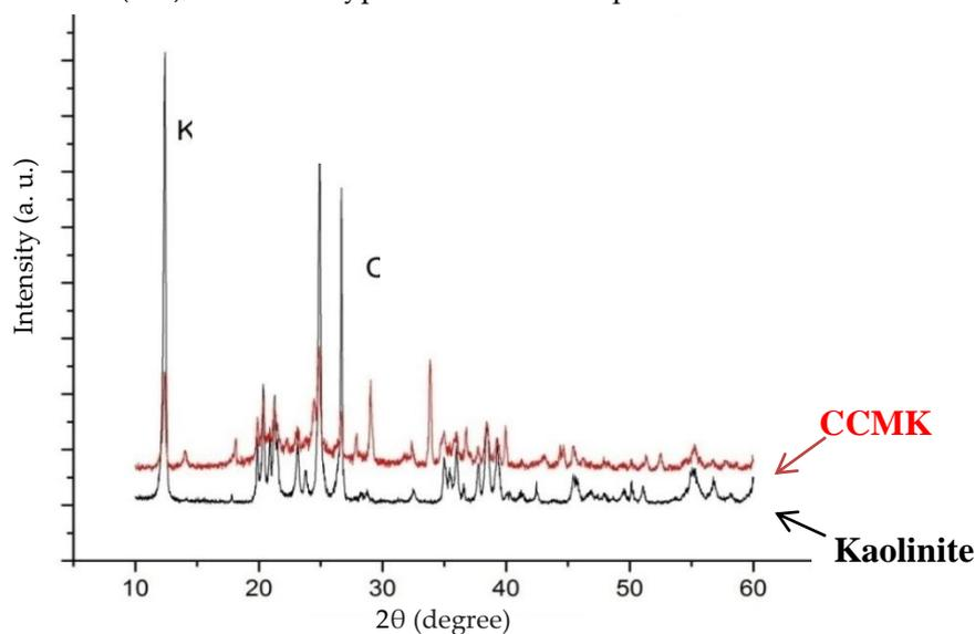
**Figure S4.** Patterns of kaolinite and choline chloride modified kaolinite.
