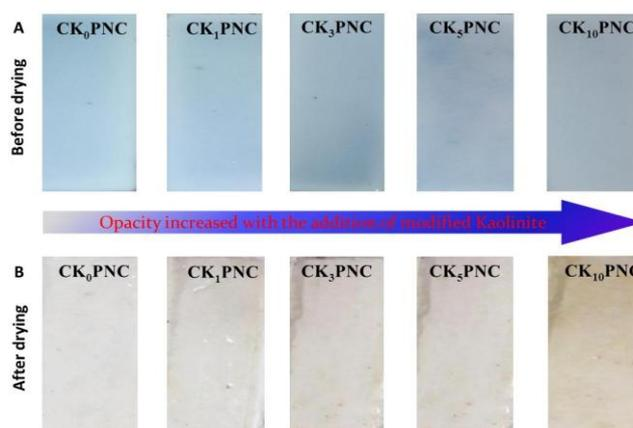
Figure S2. Camera images of nanocomposite films before (A) and after drying (B).
