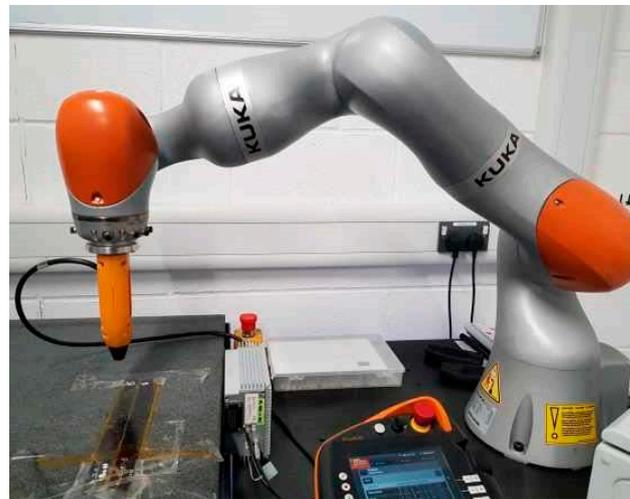
**Figure 3.** Photographs of the Kuka-iiwa collaborative robot equipped with the EddyCus EC sensor.
