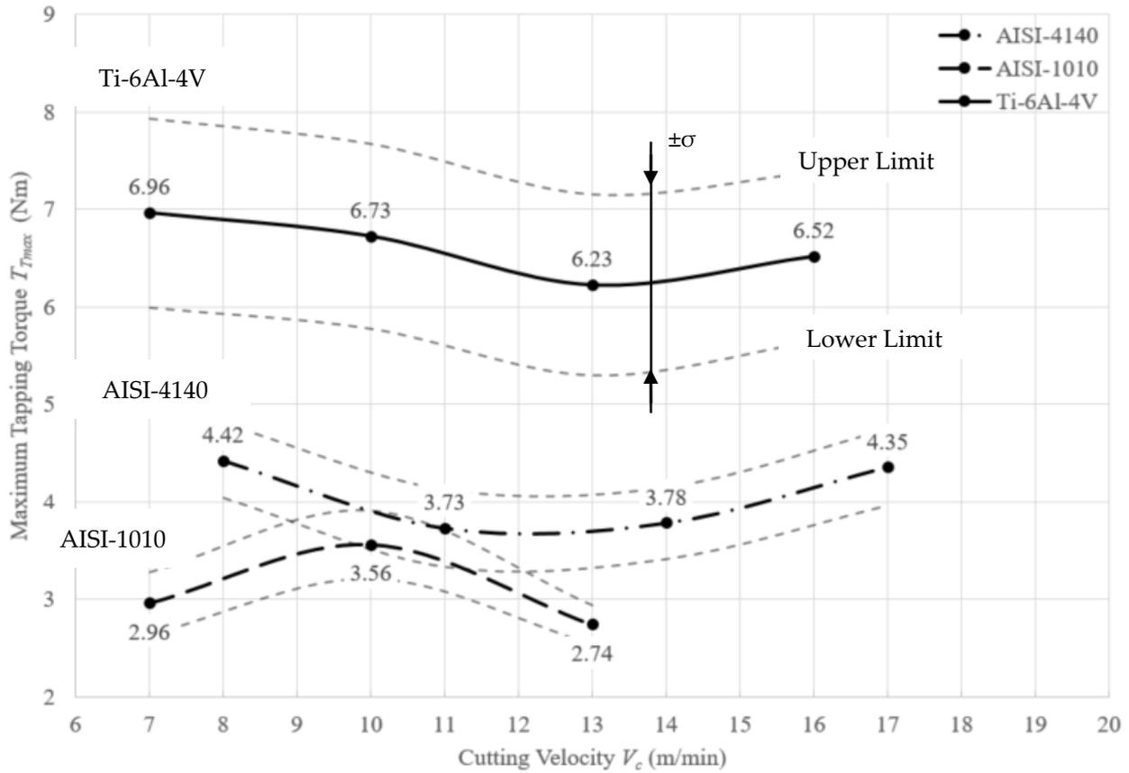
Figure 9. Maximum tapping torque for different materials and cutting speeds.
