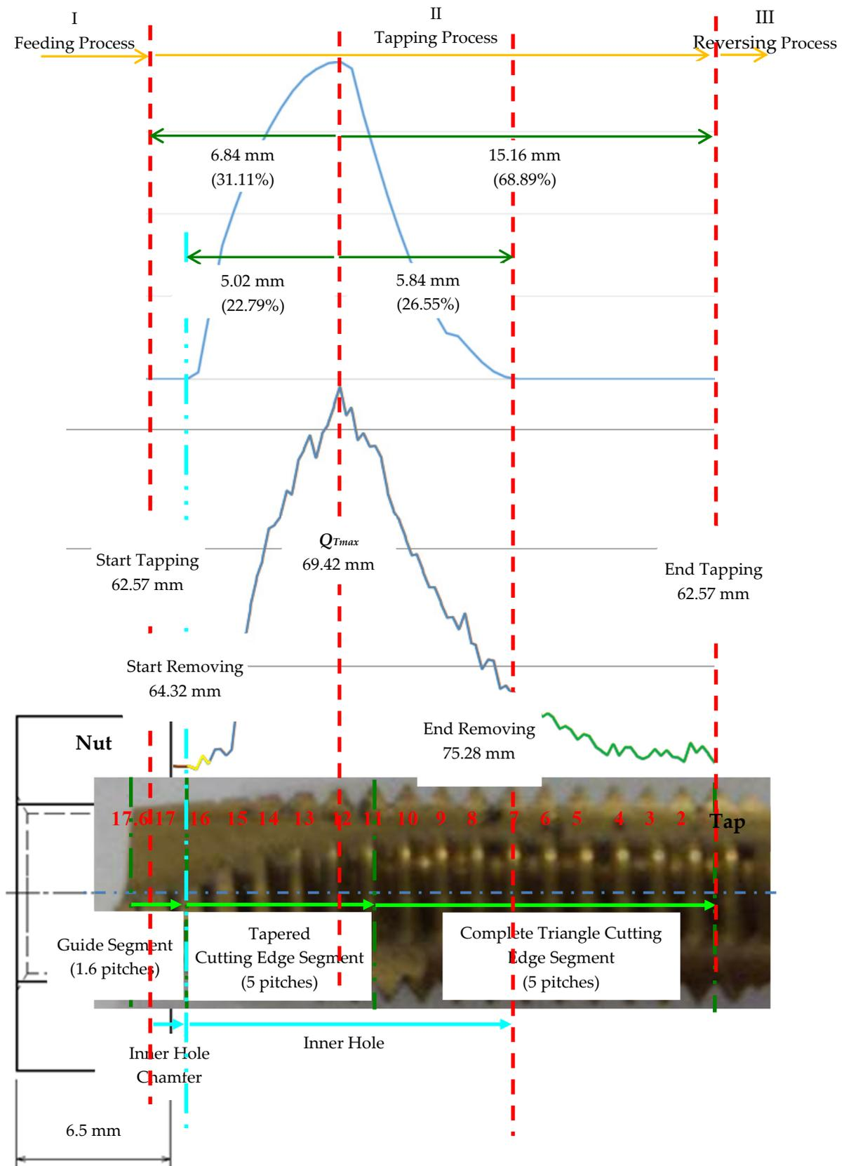
Figure 5. The characteristics of the material removal rate curve and the measured tapping torque.
