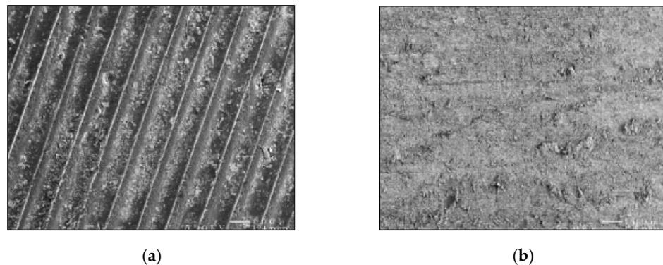
**Figure 5.** Surface finish: (a) before and (b) after the AFF process [17].
