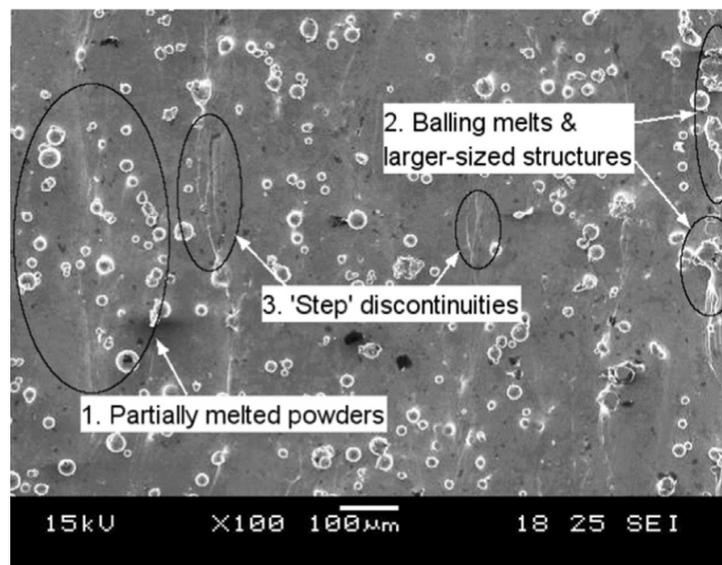
**Figure 16.** Defects that can occur in metal powder bed following AM [37].
