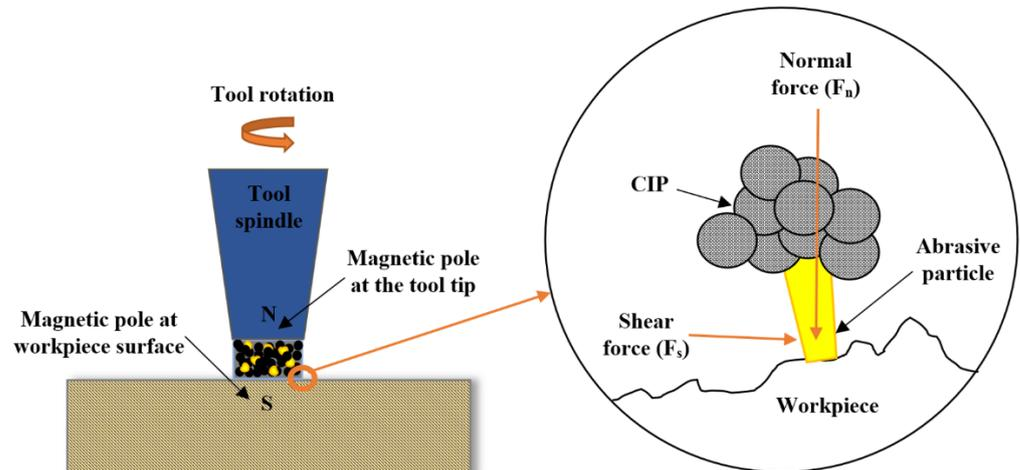
Figure 6. The BEMRF process.
