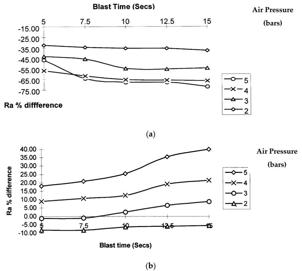
Figure 2. Surface roughness variation with respect to process parameters for: (a) aluminum oxide (b) and glass bead abrasives [13].
