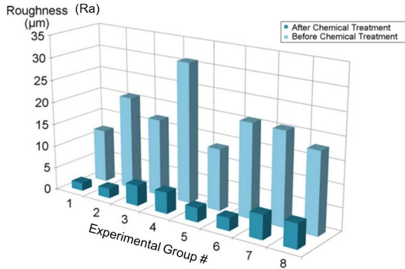
Figure 10. Surface finish improvement after chemical treatment [21].
