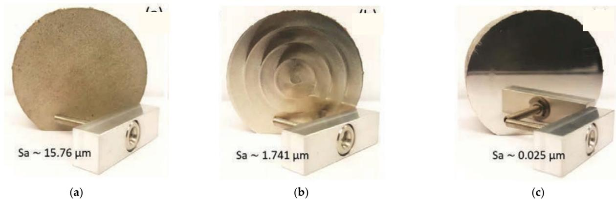
**Figure 19.** Surface finish of the part produced by powder bed laser melting: (a) without finishing; (b) after post-milling; (c) after fine abrasive finishing [97].
