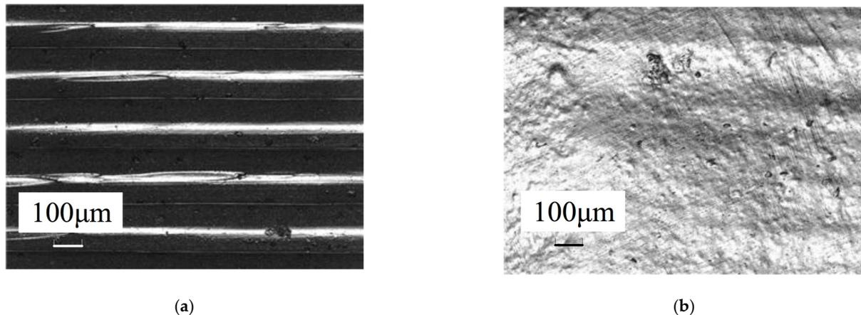
**Figure 12.** PLA parts and roughness: (a) before chemical vapor finishing and (b) after chemical vapor finishing of the surface [24].
