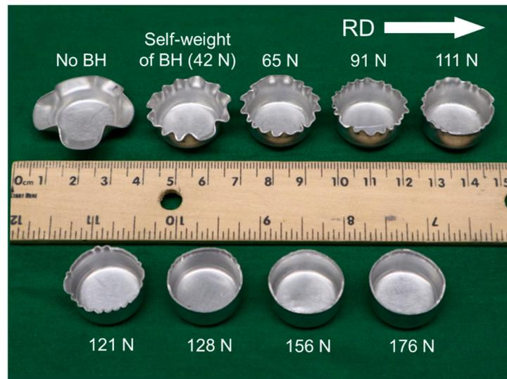
Figure 4. Aluminum AA1100-O cups (diameter 35 mm, thickness 0.51 mm) drawn under a set of BHF's ranging from zero to 176 N. Indicated in the figure is the rolling direction, RD.
