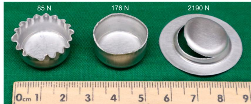
**Figure 1.** Aluminum AA1100-O cups drawn under different BHF (from left to right: wrinkled (low BHF), fully drawn (medium BHF) and torn (high BHF)). The numbers listed are the BHF.
