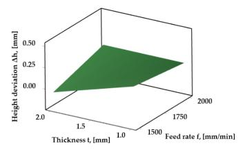
**Figure 12.** Influence exerted by the workpiece thickness t and feed rate f on the height deviation  $\Delta h$  when using a cryogenic agent ( $s_d = 0.7$  mm).
