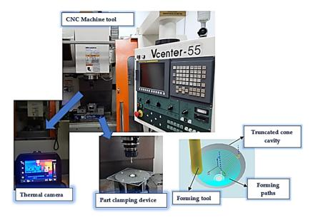
**Figure 3.** The equipment and conditions on which the single-point incremental forming process was performed.
