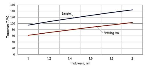
**Figure 10.** Different temperatures of the rotating forming tool and the sheet-type sample when using air as a working medium in the case of single-point incremental forming applied to polycarbonate sample (f = 1500 mm/min,  $s_d = 0.5 \text{ mm}$ ).
