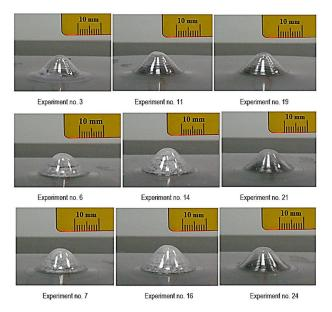
Figure 6. Examples of conical frustums obtained by single-point incremental forming.
