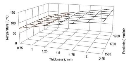
**Figure 7.** Influence exerted by the workpiece thickness t and feed rate f on the sample temperature when using coolant ( $s_d = 0.5 \text{ mm}$ ).
