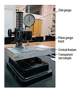
Figure 4. Setup used to measure the heights of the conical frustums.
