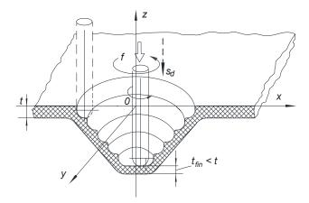
**Figure 1.** Gradual generation of the conical surface from the polycarbonate sheet by single-point incremental forming.
