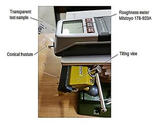
**Figure 5.** Setup used to measure the values of the roughness parameter *Ra* corresponding to the internal surfaces of the conical trunks.
