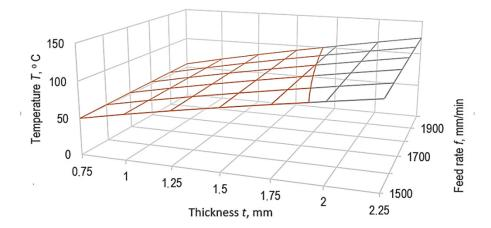
**Figure 8.** The influence exerted by the workpiece thickness t and feed rate f on the temperature of the rotating forming tool when processing in the air ( $s_d = 0.5 \text{ mm}$ ).
