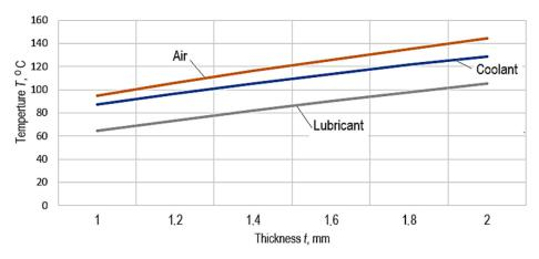
**Figure 9.** Influence exerted by the workpiece thickness t on the sample when using a coolant, air and lubricant temperature (f = 1500 mm/min,  $s_d = 0.5 \text{ mm}$ ).
