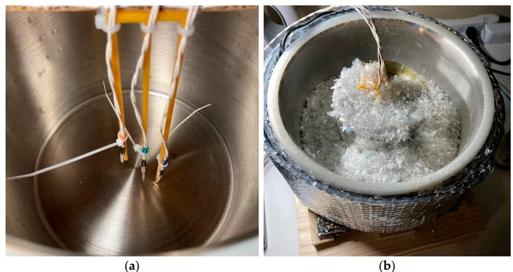
**Figure 15.** The test setup for measuring temperature gradient. (a) Three thermistors were mounted on a 3-D printed jig, mounting them 0, 25, and 50 mm above the base of the chamber. (b) For the second test, a heat sink was added in the mix of rPET to aid heat transfer throughout the material.
