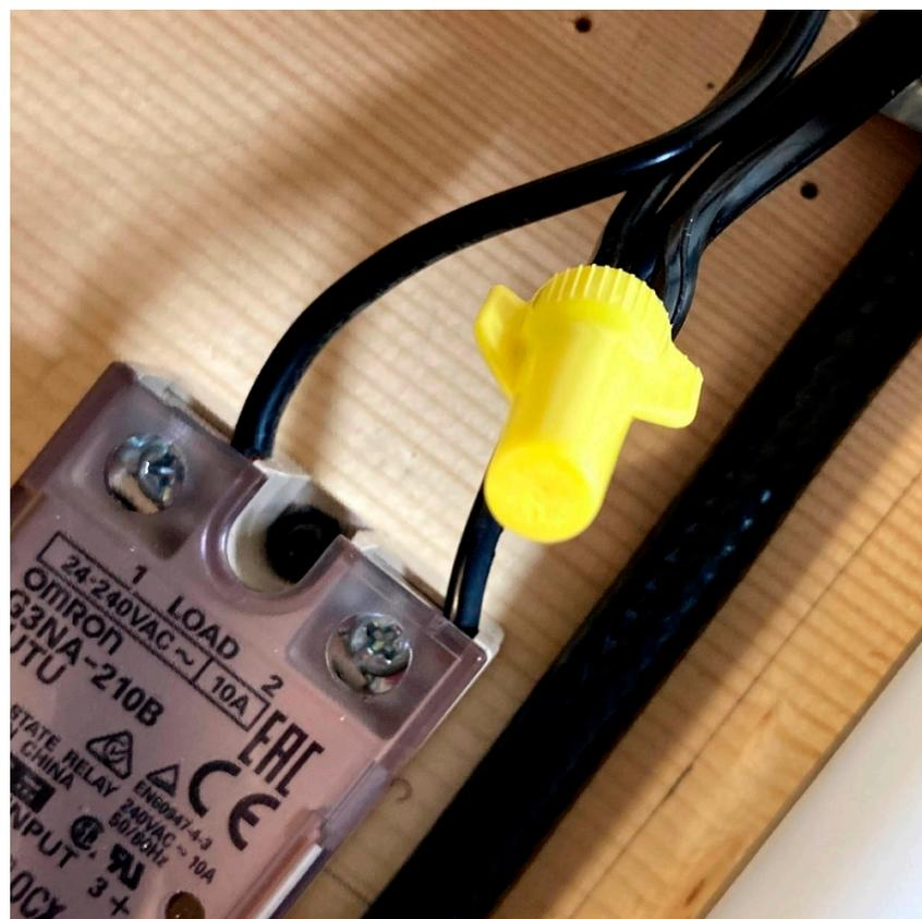
**Figure 13.** The power cable was secured into the load terminals of the relay.
