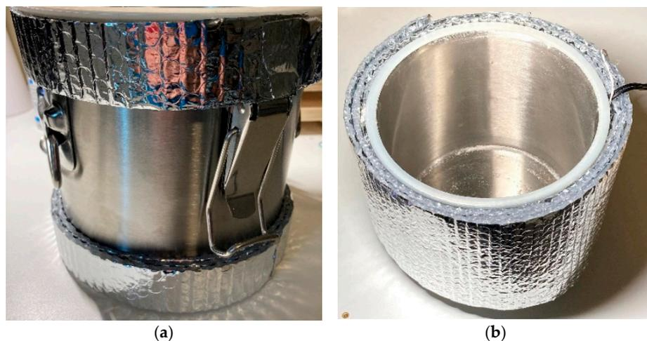
**Figure 7.** Install insulation on the chamber wall. (a) First, attach strips of insulation to build an air gap and span the protruding components on the chamber walls; (b) Next, install the large piece of insulation, fully covering the walls of the chamber.
