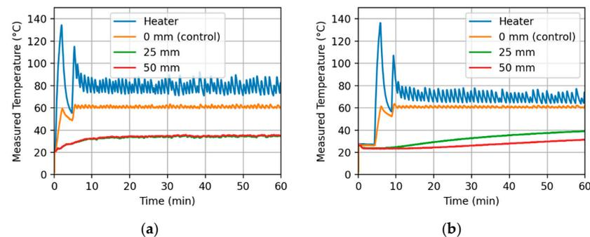
**Figure 19.** Temperature gradient measurements with the inside surface temperature used for control. (a) Chamber empty and open to the air, average heater temperature 79 °C at steady state. Note that the 25 and 50 mm curves lie on top of each other, since both are measuring air temperature inside the chamber; (b) chamber loosely packed with rPET, average heater temperature 68 °C at steady state.
