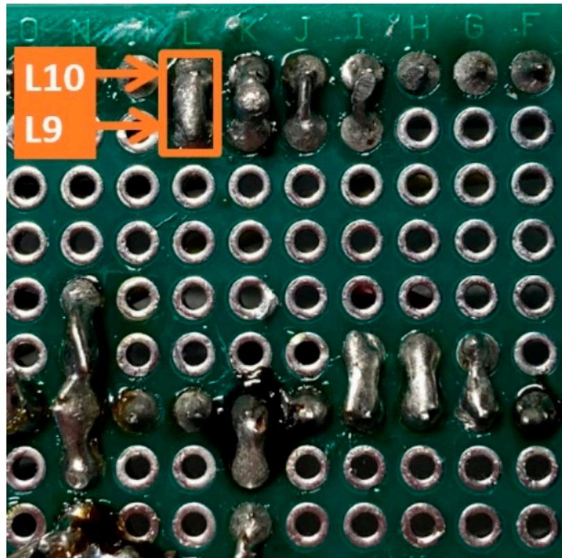
**Figure A1.** Illustration of wire solder labels. The top row is row 10, and it contained a row of header pins. A wire needed to connect to the header pin at L10. To do this, the wire was soldered into L9, then bent over onto L10 (which was already occupied by a header pin) and soldered in place. This wire would be labeled 'L9:L10'.
