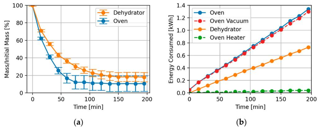
**Figure 23.** Dehydration measurements on consortium of microorganisms. (a) Percent initial mass for each sample; (b) energy consumption. The dashed oven vacuum and oven heater curves were summed to form the aggregate oven curve.
