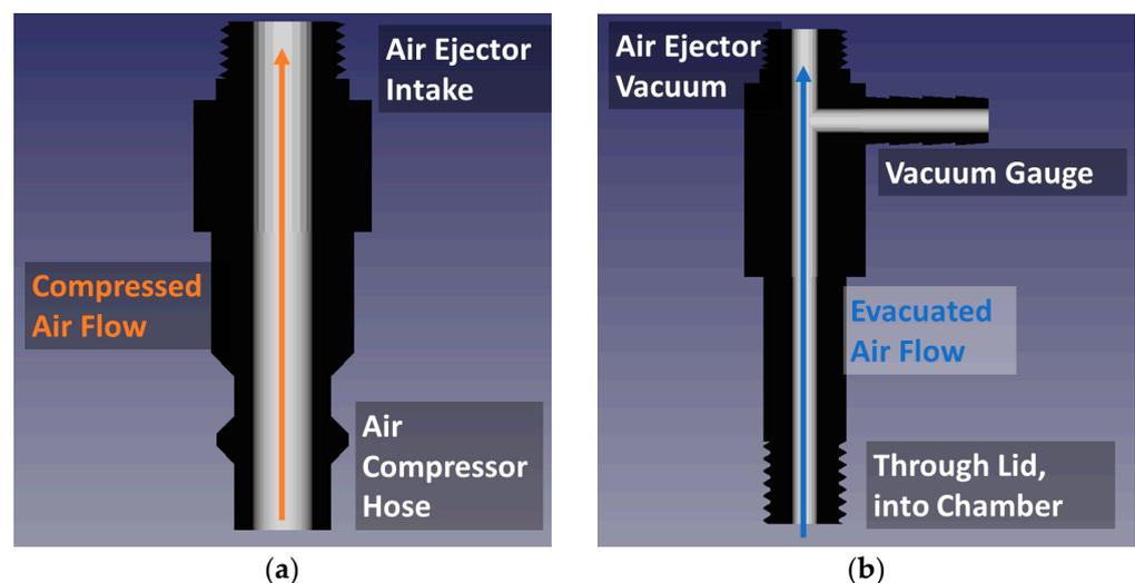
**Figure 2.** Air ejector connector cross-sections, highlighting internal geometry where air flows. (a) Intake connector, where high pressure air enters the ejector; (b) vacuum connector, where evacuated air flows from the chamber to the ejector and vacuum pressure is measured.
