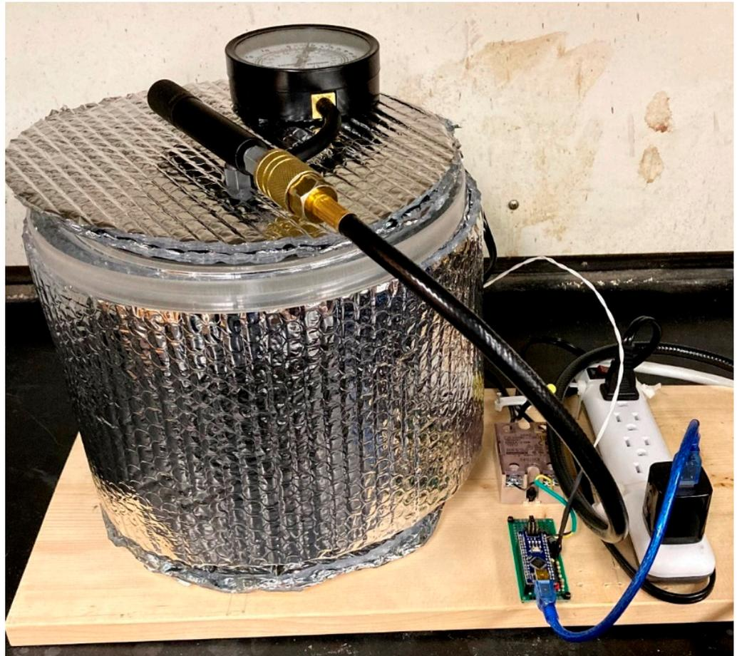
**Figure 14.** The fully assembled vacuum oven.
