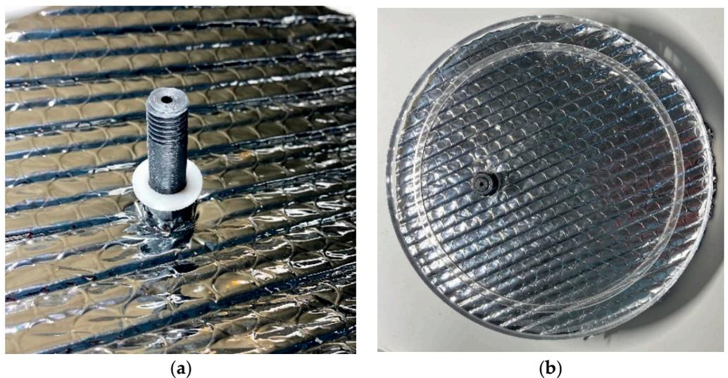
**Figure 5.** Process to connect the air ejector to the lid. Note that the photographed part is grey here, where it was orange in prior photos. (a) Feeding the vacuum connector through the insulation, then an M10 washer (nylon or rubber); (b) feeding the vacuum connector through the lid, then another washer, then secure with an M10 nut.
