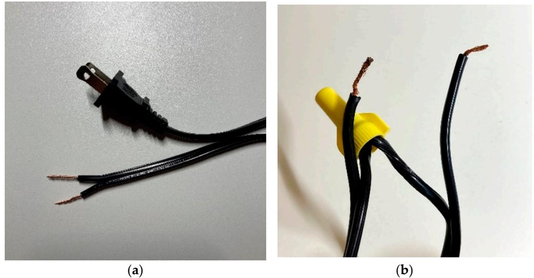
**Figure 12.** The power cable was prepared for connection to the relay. (a) First, it was cut in half. Only one wire needed to be cut, but both were cut in this case. (b) Next, one pair of wires was immediately re-joined with a wire nut.
