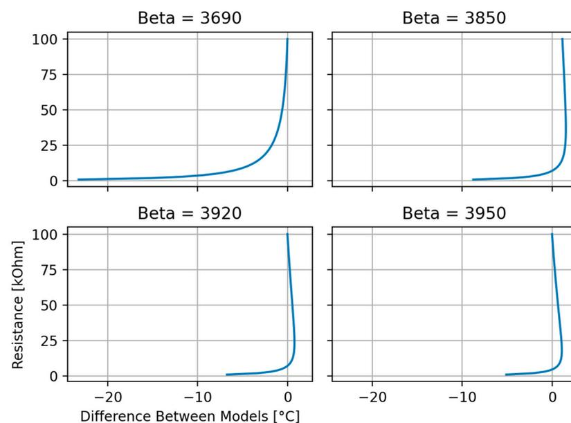
**Figure 17.** The calculated Beta values have varying accuracy as a function of resistance. These curves show that Beta of 3920 or 3950 maintain an error within 1 °C for the majority of the temperature range under assessment.
