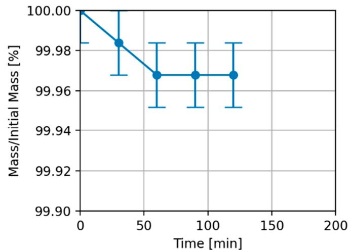
**Figure 25.** A 1 kg spool of PLA filament was dried in the vacuum oven. The change in mass was around 0.4 g, compared to the initial mass of 1245.7 g.
