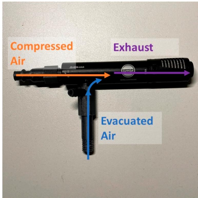
**Figure 4.** The air ejector is driven by compressed air, which creates a vacuum pressure inside the ejector, pulling air through the vacuum connector into the stream of compressed air. The exhaust is delivered into the atmosphere through a diffuser that reduces airflow noise.
