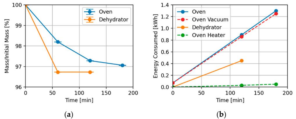
**Figure 21.** Dehydration of large (350g) samples of rPET. This test was cut short because it clearly indicated that the vacuum oven could not manage the large mass of plastic and water. (a) The percentage of initial mass as a function of time. (b) The energy consumption of each device. The energy consumption of the vacuum is shown as an aggregate of the two components, the heater and the vacuum.
