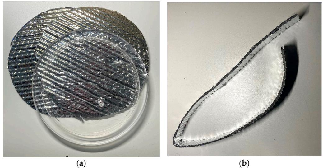
**Figure 1.** Insulation was cut to fit the specific vacuum chamber that was purchased. (a) Circles of insulation to cover the base and lid; (b) a strip of insulation to be wrapped around the circumference of the chamber to build an air gap.
