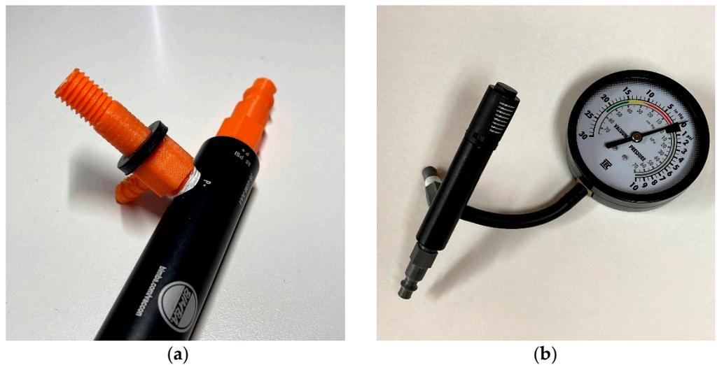
**Figure 3.** Assemble the air ejector. (a) Thread the 3-D printed connectors into the air ejector, using PTFE tape if necessary; (b) attach the vacuum gauge to the hose barb. Note that the same parts were printed in orange (left) and grey (right) PLA.
