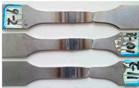
**Figure 12.** Shapes and fracture position of tensile specimens after stretching.
