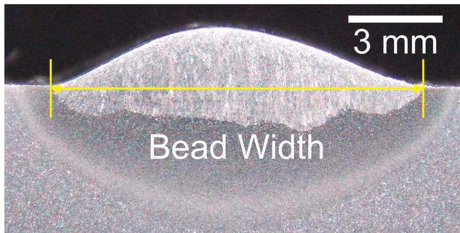
Figure 11. Test specimen optimized in relation to the smallest width of the weld bead.
