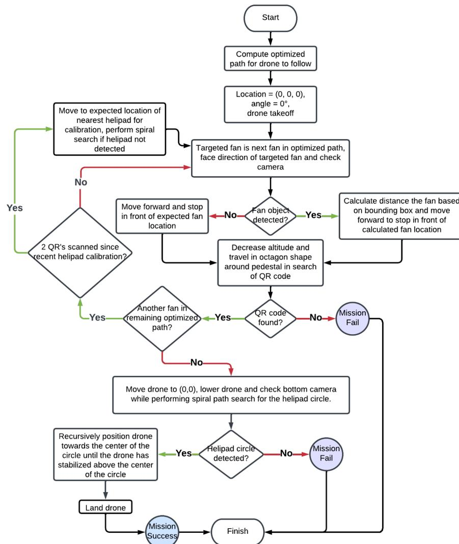
**Figure 13.** Flowchart of the early version of the traveling salesman functionality in which the real-time recorded drone location would be updated by centering over the known location of helipads.
