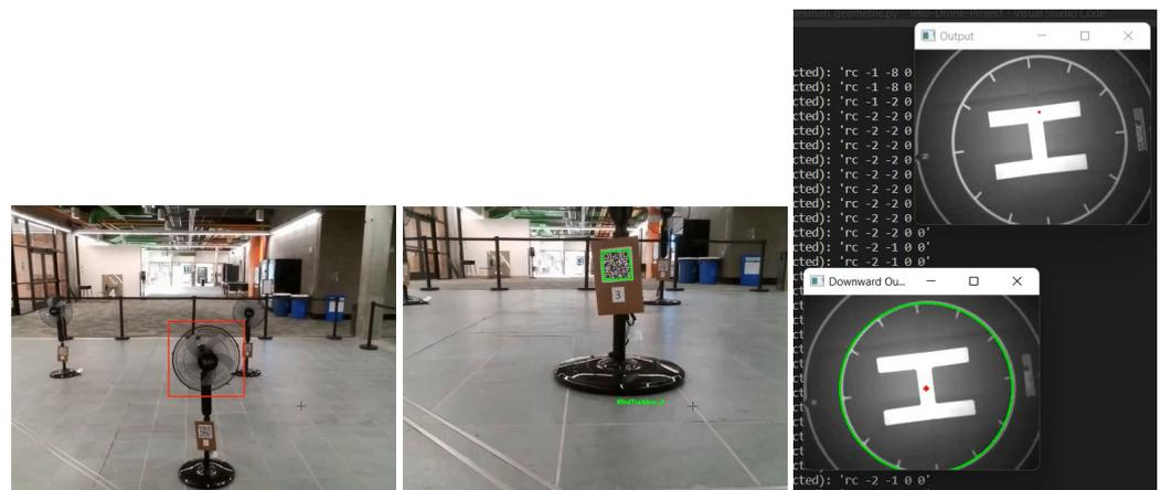
**Figure 10.** From left to right the OpenCV's rectangle function is applied to Haar detection boundaries for the red bounding boxes. The QR code is used for target verification and is read by the Python library 'pyqrcode'. Using frames from the bottom camera live stream window, the Hough transform function is applied to detect the helipad circle and displays the modified image in a new window.
