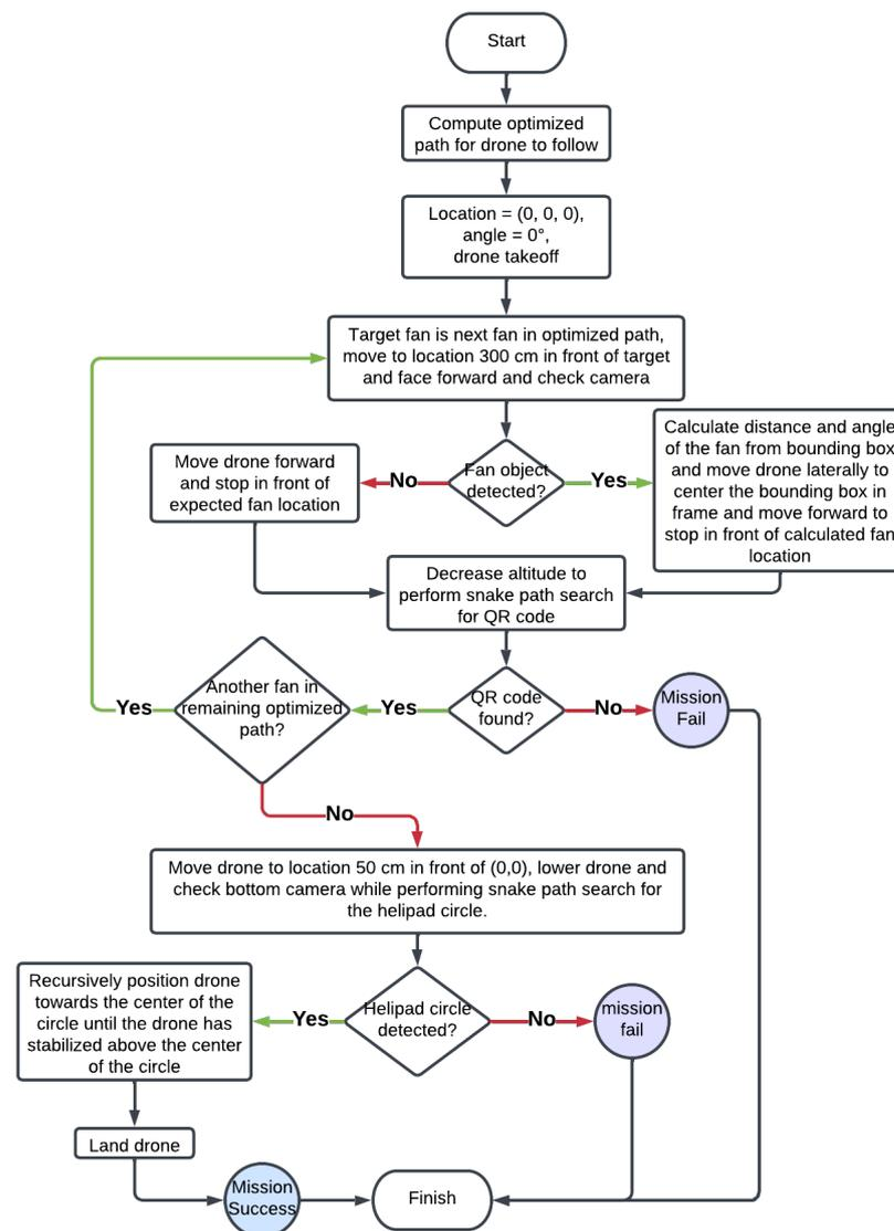
**Figure 21.** Flowchart of the revised traveling salesman functionality, where calibration is no longer conducted via helipads but through object detection of the known fan locations and QR codes confirming each location.
