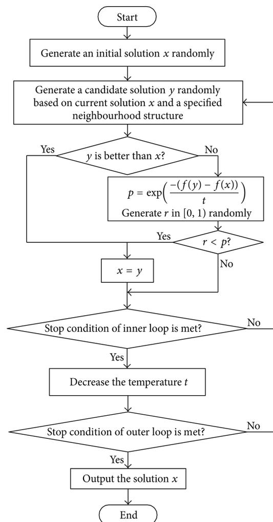
**Figure 3.** Flowchart of list-based simulated annealing (LSBA) algorithm [38].
