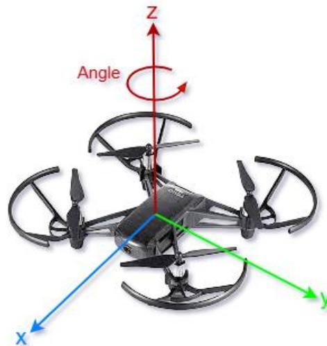
**Figure 1.** DJI Tello EDU quadcopter equipped with a front-facing camera (used for object detection) and bottom camera (used for vision position system) with the coordinate system of the body frame.
