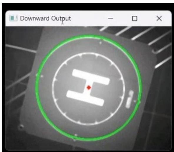
**Figure 20.** The drone recursively follows computed travel vectors until the frame's center is near the circle center.
