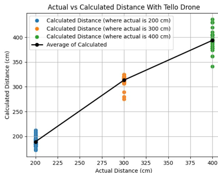
**Figure 8.** Illustration of the relationship between the actual and calculated distance based on object detection bounding boxes.
