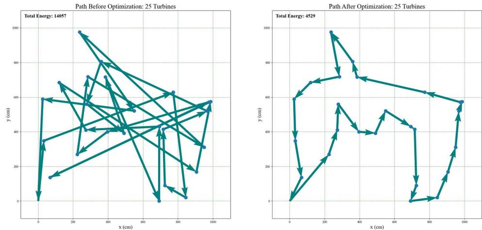
**Figure 4.** A demonstration of the heuristic simulated annealing on a cyclic path of 25 randomly selected points. The arrows indicate the direction the drone is to travel in the exploratory area.
