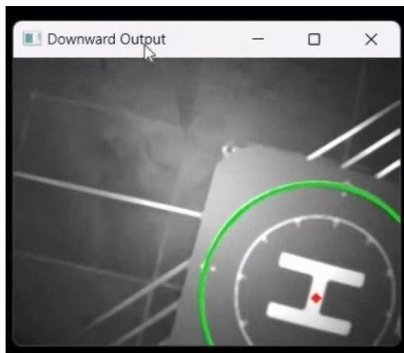
**Figure 19.** Hough transform for detecting the circle and a travel vector from the frame's central pixel to the circle's center pixel.
