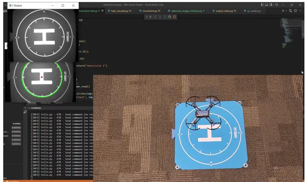
**Figure 7.** An example showing the drone centers over the helipad using Hough transforms to provide feedback on the drone's current position.
