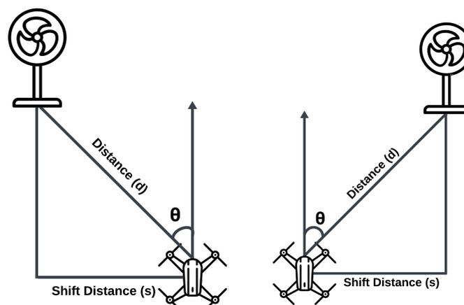
**Figure 9.** The aerial view of two cases used for calculating  $d$ ,  $\theta$ , and  $s$ . The left/right diagram refers to the case where the  $x$ -center of the bounding box is less/greater than half of the pixel width of the image.
