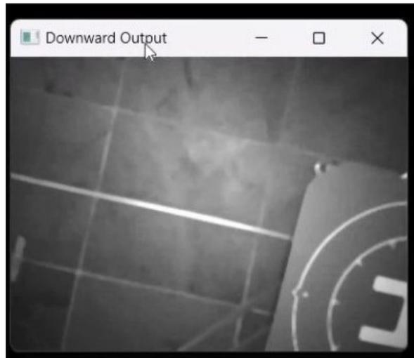
**Figure 18.** Although the helipad is in the frame, the exploration path continues since no circle is detected.
