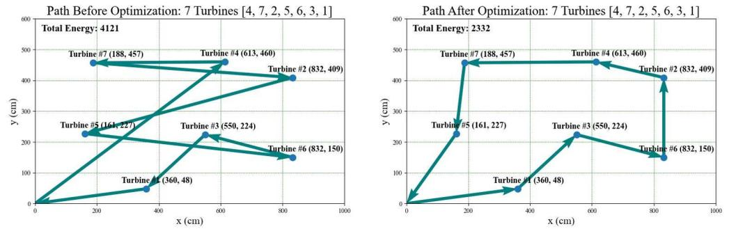
**Figure 11.** A demonstration of the heuristic simulated annealing for 7 randomly ordered fans used in experiments where fan identification is labeled.
