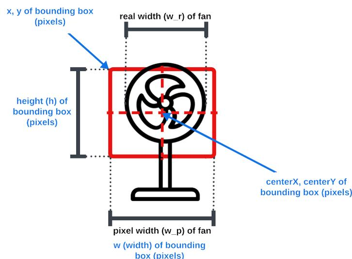
**Figure 6.** The parameters returned from Haar cascade object detection are used to calculate the  $x/y$  distance and angle of the fans for the drone. The size and center of the bounding box may not always represent the precise location of fans (turbines), as demonstrated in the recorded videos.
