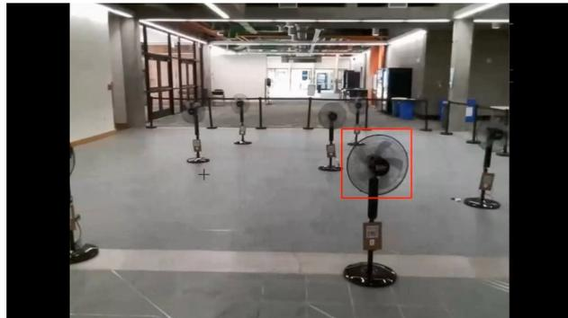
**Figure 15.** The bounding box center pixel is deemed too far from the frame's center pixel so that a lateral shift can be performed.
