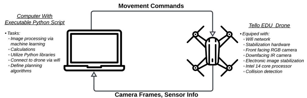
**Figure 2.** Flowchart depicting the communication cycle between the local computer with Python scripts and DJI Tello EDU drone.
