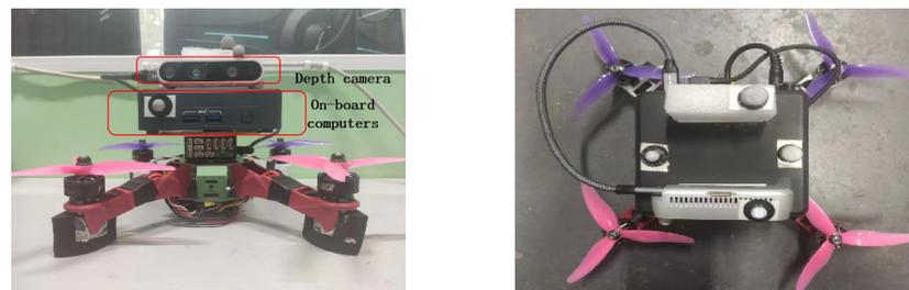
**Figure 15.** Physical drone hardware configuration.
