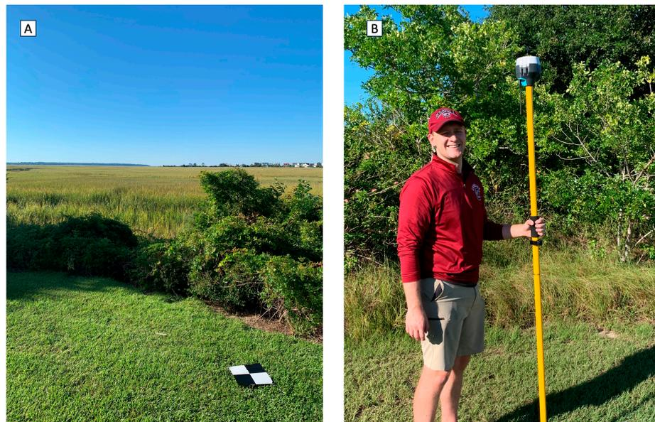
**Figure 2.** (A) An example of a black and white GCP surrounding the area of interest. (B) The EMLID reach RS2 rover pole collecting data for the GCPs.
