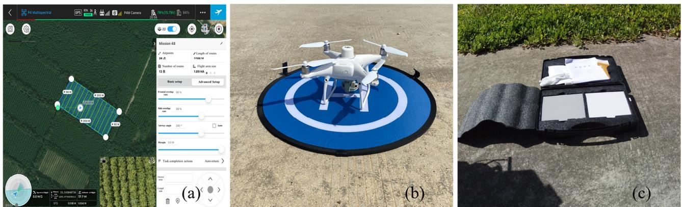
**Figure 3.** (a) Flight route (green line) and parameters, (b) DJI Phantom 4 multispectral (P4M), (c) Diffuse reflectance board (right).
