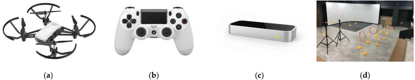
**Figure 1.** Apparatus of this study: (a) Drone (DJI's Tello), (b) Gamepad (Sony DualShock 4), (c) 3D controller (Leap Motion), and (d) setup of the experiment place with a 12-camera motion-capture system (OptiTrack).
